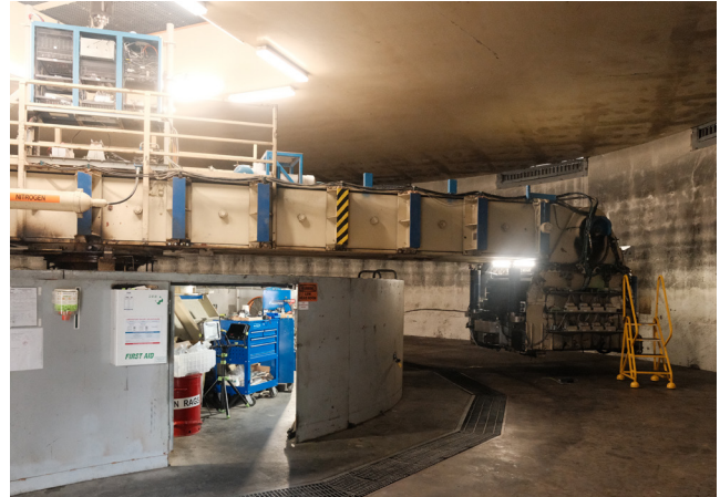
Image 1: The 9-m radius centrifuge (Center for Geotechnical Modeling, UC-Davis).
