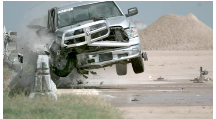
Image 4: Test 616811-01-4 PCC Bolted Median Configuration with 5 inch embedment 2023_09_29
