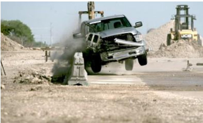
Image 2: Test 616811-01-2 PCC Bolted Roadside Configuration 2023_03_13
