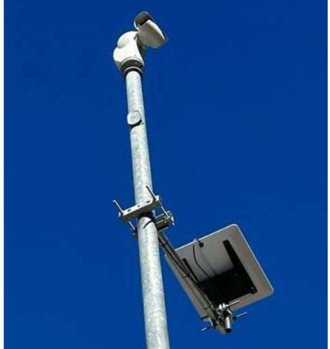
Image 3: Starlink high-performance flat antenna after installation – Image Source – AHMCT
