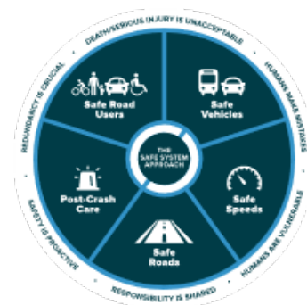
Image 2: Safe System Approach(SSA)Wheel Diagram of the Five SSA Elements and Six SSA Principles
