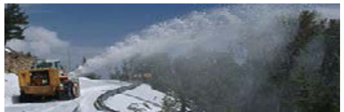
Image 1: Rotary blower removing snow from roadway
