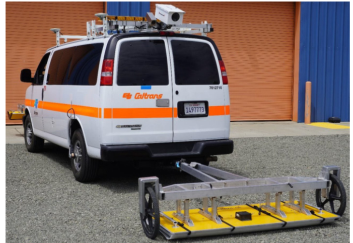
Image 1: The Caltrans NDE vehicle (rear view, showing GPR antenna and trailer). The IR and B/W camera housings are mounted at the NDE vehicle rear on top of the roof.
