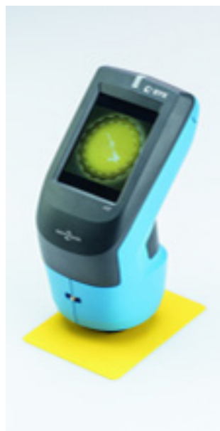
Image 3: Spectrometer to measure daytime chromaticity
