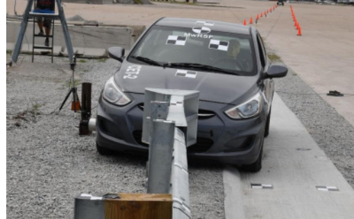
Image 5: Crash Test CET-2 (Test 3-32) Pre-Test
