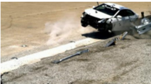
Image 3 and 4: Crash Test CET-1 (Test 3-30) During Impact
