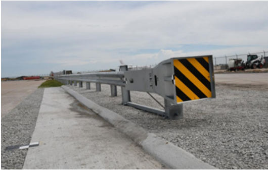
Image 1: End Terminal with 4-inch Curb Prior to Test
