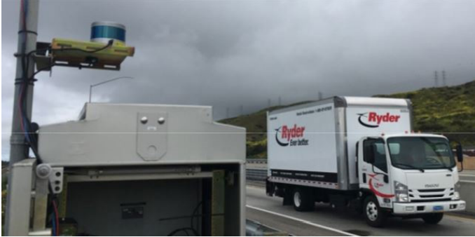
Image 2: A Velodyne LiDAR detector records a point-cloud image of a passing truck on SB I-5 at San Onofre
