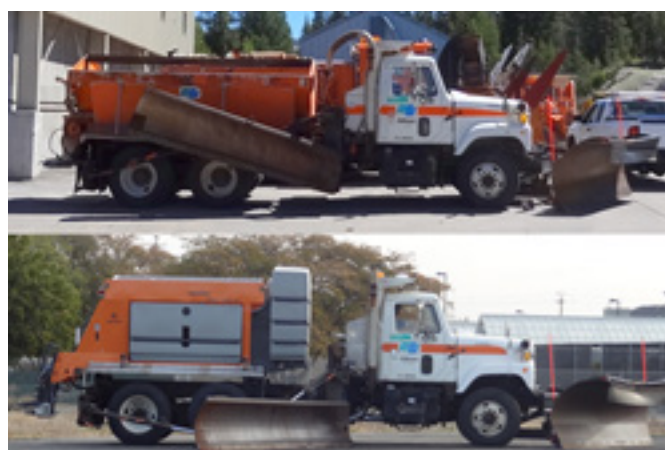
Pictured on top is the Henderson V-box sander/spreader, on bottom is the Epoke sander/spreader with directional cast.
