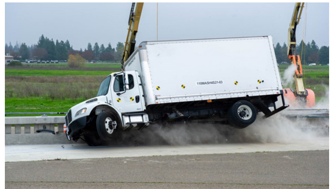
Image 7: 10000S (Single-Unit Truck) test on Type 86H Concrete Barrier Rail Looking East
