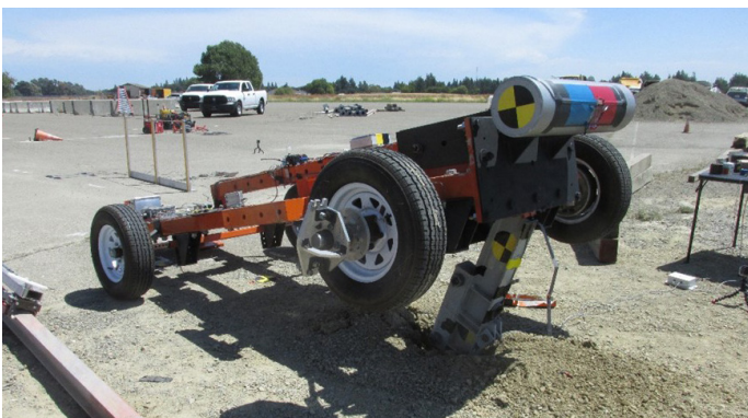
Image 3: Test 610MASH0B25-03: Dynamic Bogie Test.
