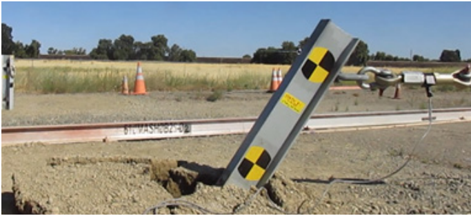
Image 1: Static Test of New Compaction Method 1.
