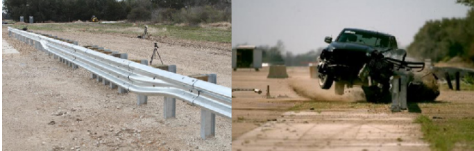
Image 2: GUARDRAILS: MASH TL-3 Testing of a Thrie-Beam Guardrail System at a Fixed Object
