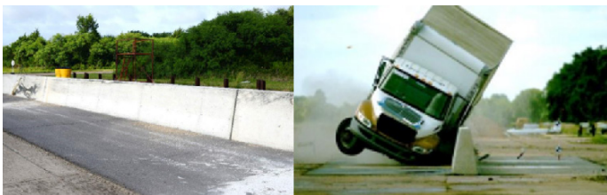
Image 4: CONCRETE BARRIERS: MASH Test 4-12 on Keyed-in Single-Slope Barrier with 40-ft Segment Length
