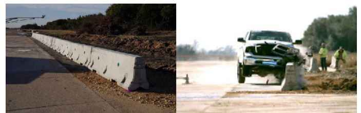
Image 1: CAL F-23 Portable Concrete Barrier: Design and Testing of MASH TL-3 Compliant Anchored F-shape Portable Concrete Barrier System with Vertical Anchors
