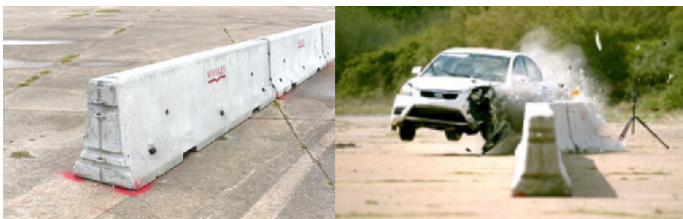
Image 5: PORTABLE CONCRETE BARRIERS: MASH Testing of Free-Standing and Pinned Temporary Concrete Barrier
