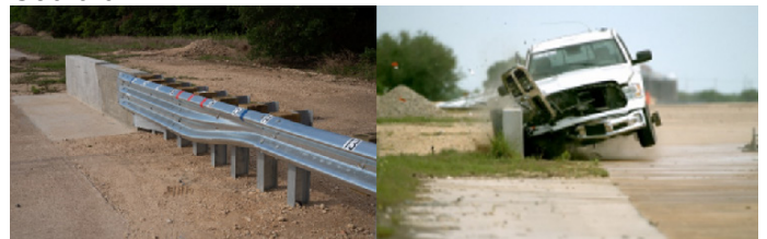
Image 7: TRANSITIONS: MASH Test 3-21 Evaluation of Short W-Beam Transition
