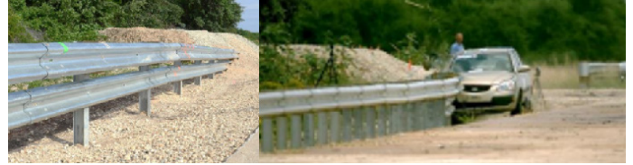
Image 6: TERMINALS: MASH Tests 3-34 and 3-35 on the 31-inch Buried-in-Backslope Terminal Compatible with MGS Guardrail
