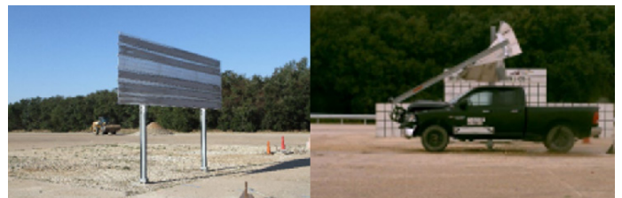
Image 8: SUPPORT STRUCTURES: Testing and Evaluation of Large Sign Slipbase Support on Slope
