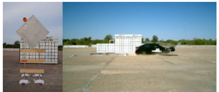
Image 9: WORK ZONE TRAFFIC CONTROL DEVICES: Evaluation of Type III Barricades with Mounted Signs
