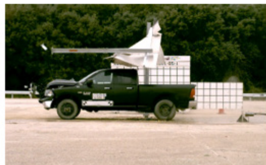
Image 1: Pooled Fund Example Project: MASH TL-3 Testing and Evaluation of Large Sign Slipbase Supports (impact sequence)
