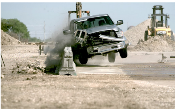
Image 2: Test 616811-01-2 PCC Bolted Roadside Configuration 2023_03_13
