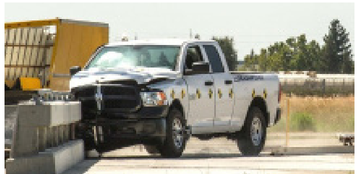
Image 4: Type 85 Bridge Rail: Pickup Truck Impact
