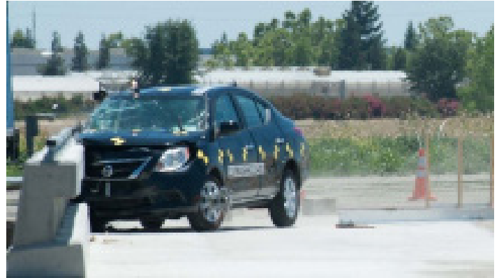
Image 3: Type 85 Bridge Rail: Small Car Impact
