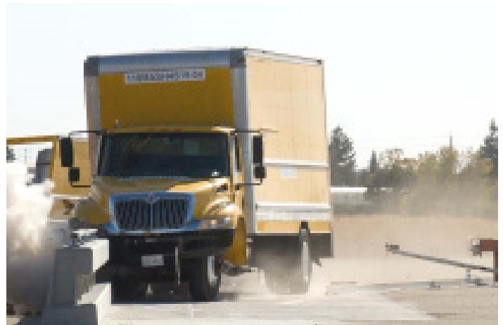
Image 5: Type 85 Bridge Rail: Van Body Impact
