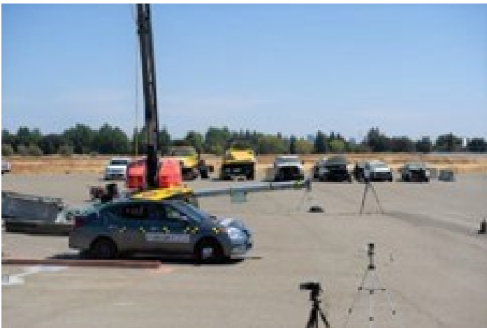
Image 5: TEST 410MASH3C22-01 Small Car 19 MPH Impact (September 14, 2022)
