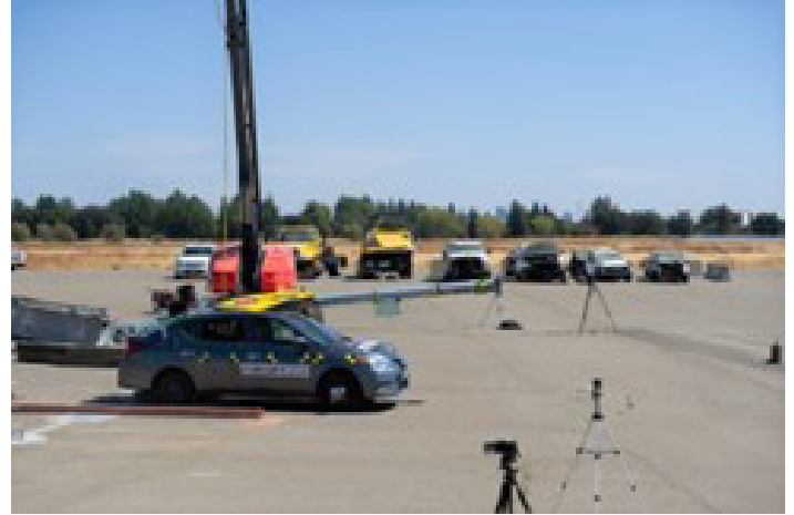
Image 6: TEST 410MASH3C22-01 Small Car 19 MPH Impact (September 14, 2022)
