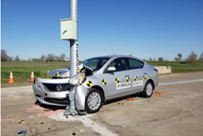
Image 4: TEST 410MASH3C20-01 Small Car 19 MPH Impact (February 26, 2020)
