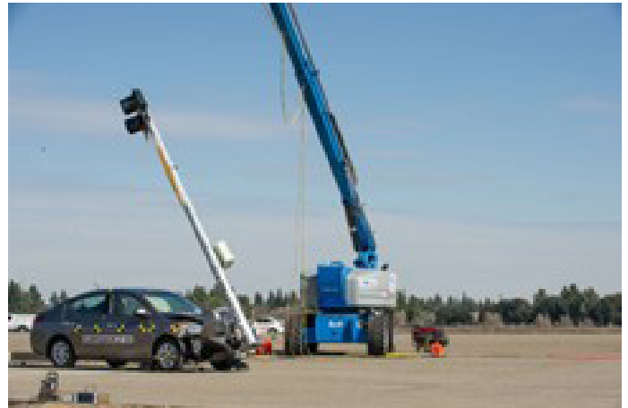
Image 3: Test 430MASH3C17-01 Small Car 31 MPH Impact (March 7, 2018)
