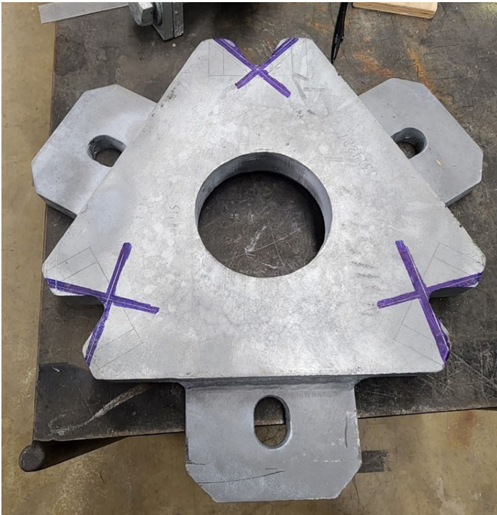
Image 5: TYPE 15-FBS SLIPBASE MODIFICATIONS – INCREASE NOTCH ANGLE FROM 60° TO 90°
