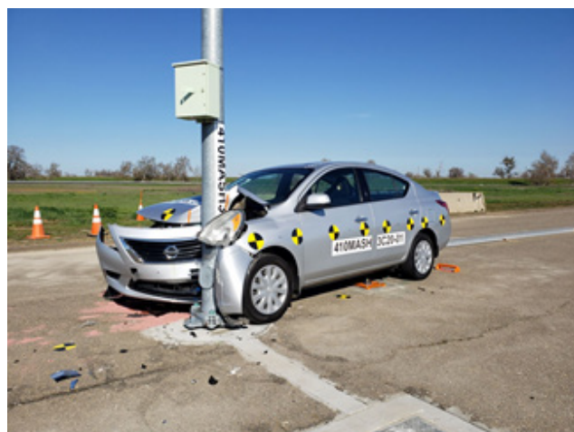
Image 4: TEST 410MASH3C20-01 Small Car 19 MPH Impact
