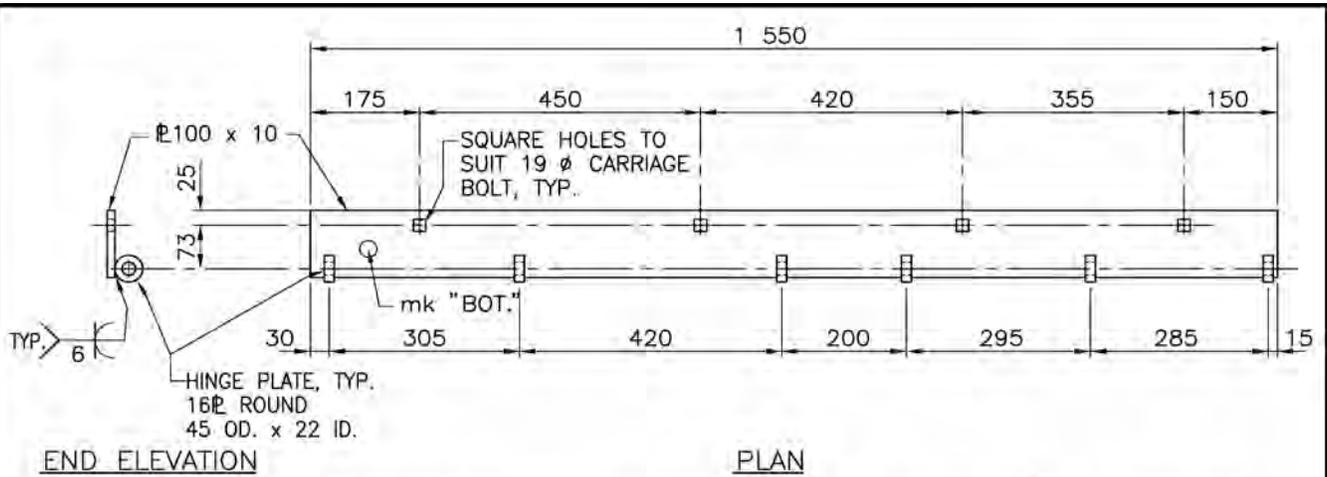
ONE REQUIRED – MOUNTING  $\bar{\bar{P}}$  – Mk. A1<sup>R</sup> (SHOWN)
