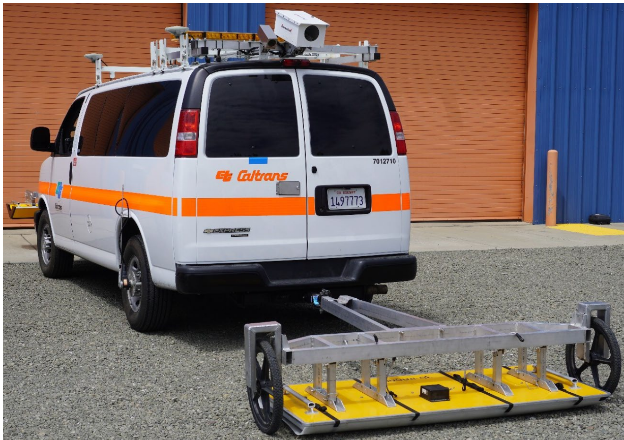
Figure 1: The Caltrans NDE vehicle. In project deployment, either the front or rear GPR antenna is used. The IR and B/W housing is mounted at the NDE vehicle rear on top of the roof
