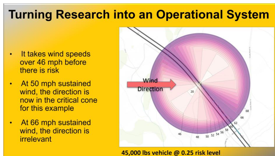
Figure 4. Variables Impacting the Weight-Based Wind Closure System
