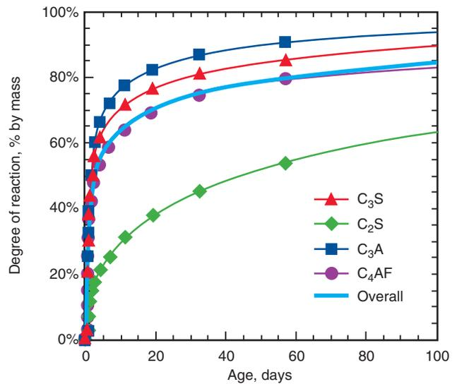
**Figure 3-30.** Relative reactivity of cement compounds. The curve labeled “Overall” has a composition of 55%  $C_3S$ , 18%  $C_2S$ , 10%  $C_3A$ , and 8%  $C_4AF$ , an average Type I cement composition (Tennis and Jennings 2000).
