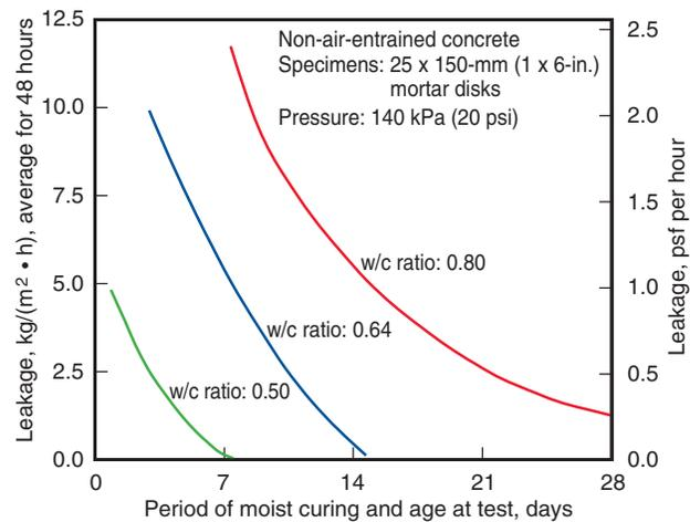
**Figure 9-30.** Effect of water-cement ratio (w/c) and curing duration on permeability of mortar. Note that leakage is reduced as the water-cement ratio is decreased and the curing period increased (McMillan and Lyse 1929 and PCA Major Series 227).
