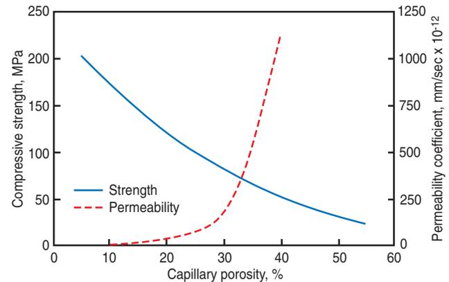
**Figure 11-5.** Both compressive strength and permeability are related to the capillary porosity of the cement paste, but in different ways. Above about 30% porosity, the permeability increases dramatically (adapted from Powers 1958).
