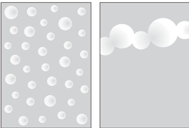
**Figure 11-3.** Porosity and permeability are related but distinct. The two hypothetical materials above have about the same porosity (total volume of pores), but very different permeabilities. Discrete pores have almost no effect on permeability, while interconnected pores increase permeability.
