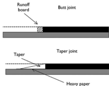
Figure 6.11 Transverse joints.
