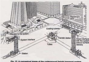
Fig. 13 A conceptual image of the underground freight transport system
