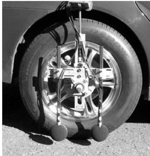
Figure 1 Dual probe vertical OBSI setup (2)
