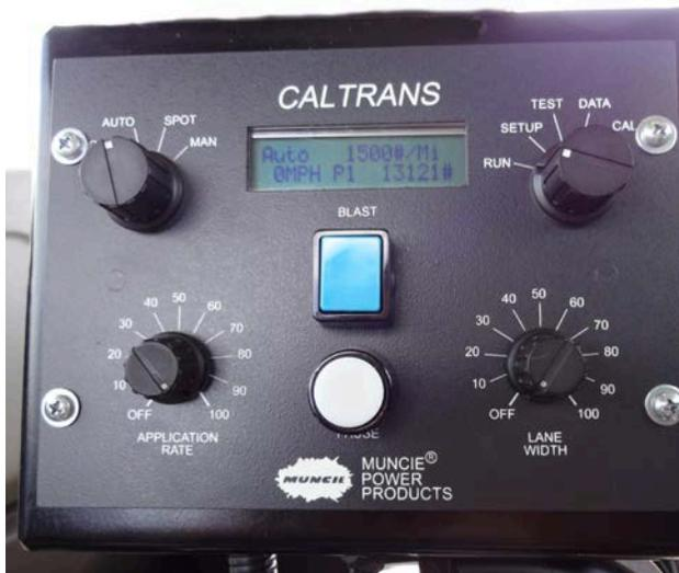
**Figure 39. Caltrans Standard Muncie Spreader Controller (Caltrans)**
