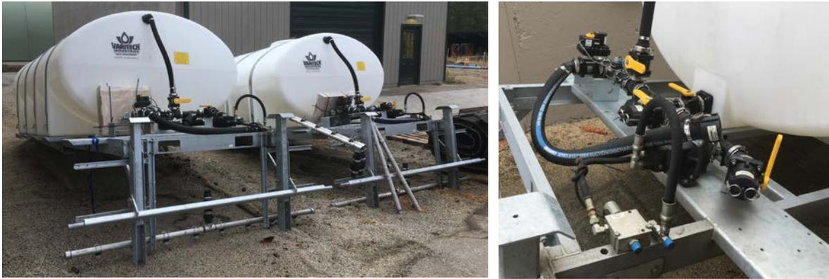
**Figure 20. VariTech Industries Liquid Application Slip-In Systems (Caltrans, South Lake Tahoe)**
