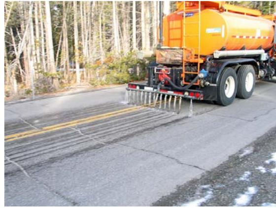
Figure 3. Brine Tanker Anti-Icing (Caltrans)
