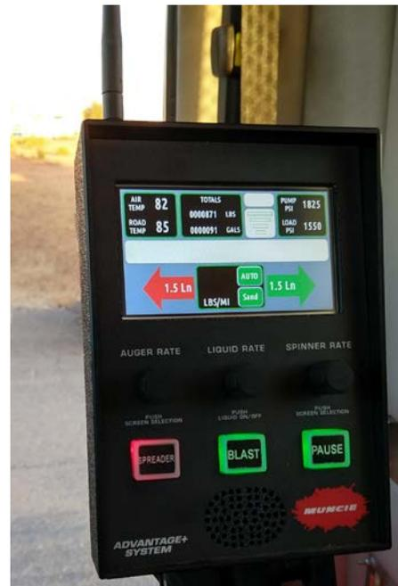
**Figure 40. Muncie Advantage Plus Spreader Controller (Caltrans)**
