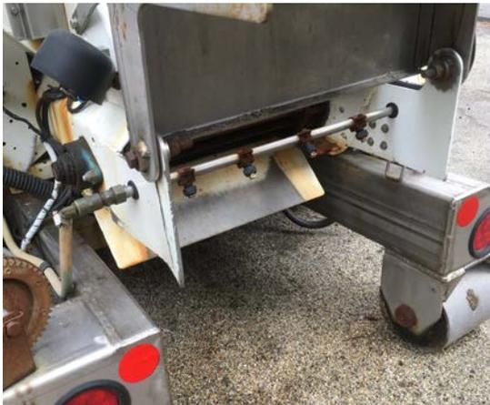
Figure 25. Basic Spreader Spray Pre-Wet System (Caltrans South Lake Tahoe)
