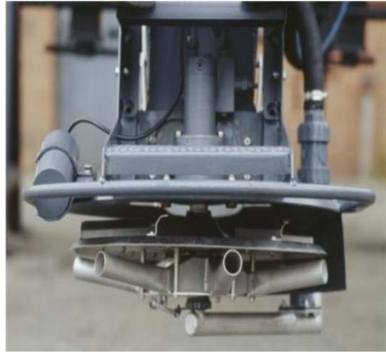
**Figure 17. Liquid Spinner (Epoke)**
