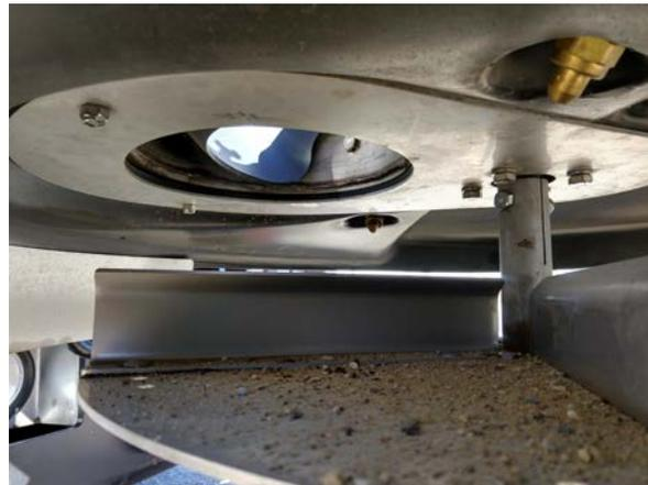
Figure 26. Henderson FRS Direct-Cast™ Pre-Wet Nozzles (Caltrans)
