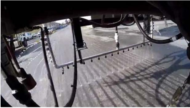
**Figure 14. Direct Brine Application Spray Nozzles (North Dakota DOT)**
