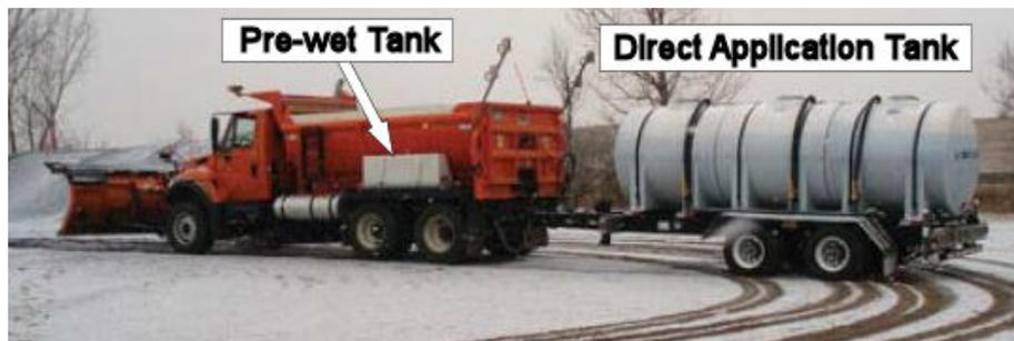
**Figure 8. Truck Pre-Wet Spreader and Direct Brine Application Trailer (North Dakota DOT)**
