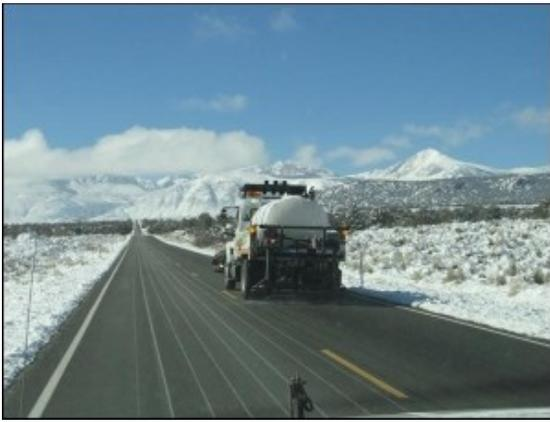
Figure 2. Highway Anti-Ice Treatment (Caltrans)
