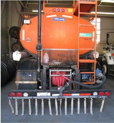
**Figure 16. Kingvale Tanker Truck with Liquid Drip Tubes (Caltrans)**
