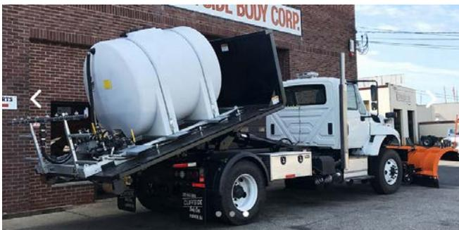
**Figure 9. Snow Plow with Roll-Off Body Mounted Anti-Ice Spray System (Cliffside Body Corp.)**
