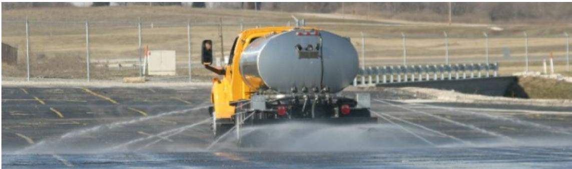
**Figure 18. Multi-Lane Brine Spraying**
