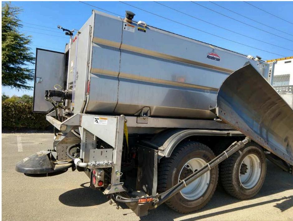
**Figure 43. Caltrans Henderson FRS Truck Mounted**
