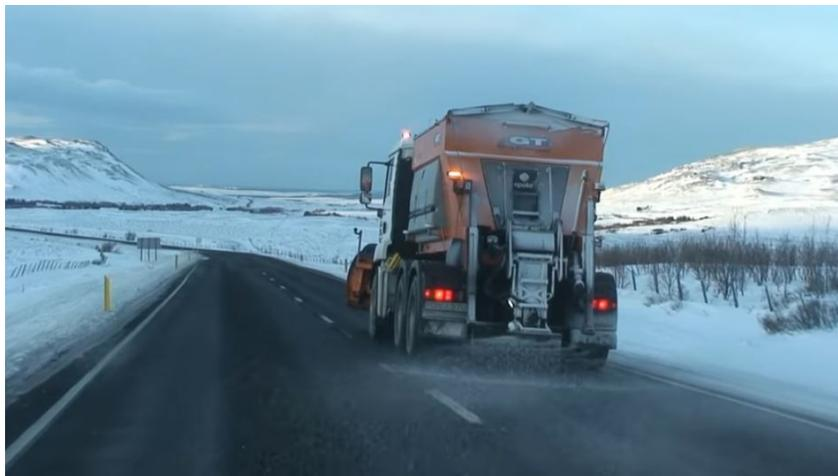
Figure 4. Sanding with Pre-Wet Treatment (Epoke)
