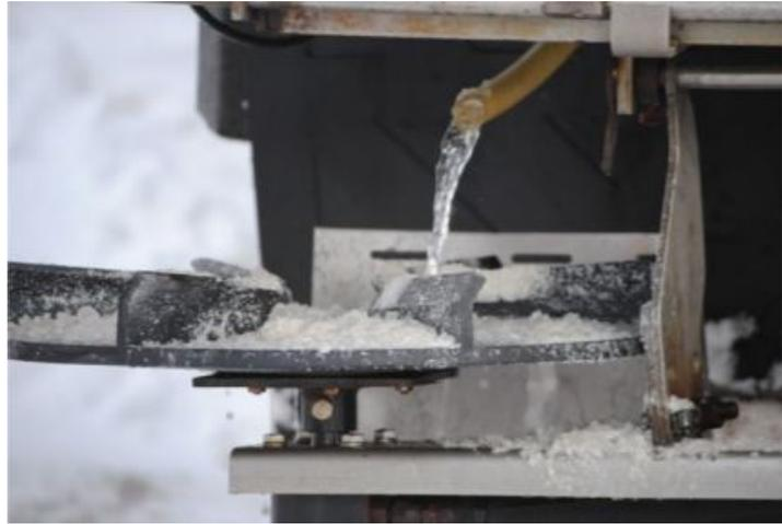
Figure 24. Basic Spreader Flood Pre-Wet System (Minnesota DOT)
