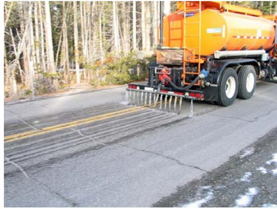
Figure 3. Brine Tanker Anti-Icing (Caltrans)
