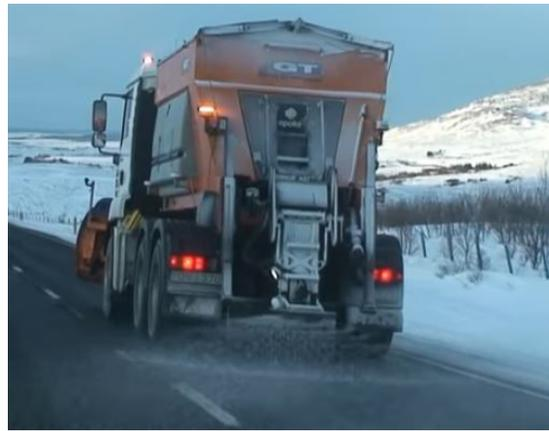
Figure 28. Epoke Pre-Wet Application (Epoke)
