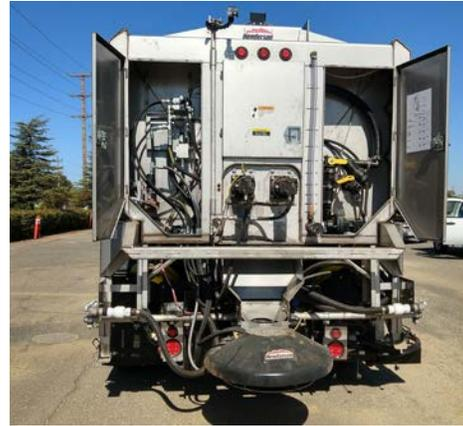
Figure 31. Henderson FRS Direct-Cast™ Pre-Wet (Caltrans)
