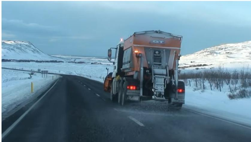
Figure 4. Sanding with Pre-Wet Treatment (Epoke)
