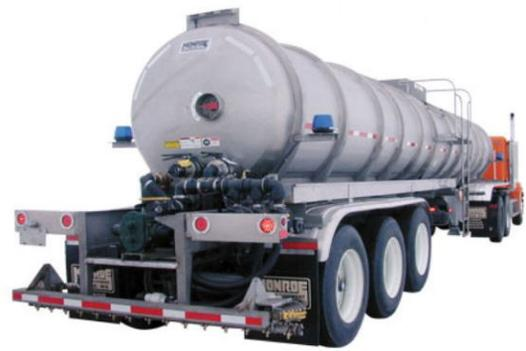
**Figure 12. Semi-Trailer-Mounted Anti-Ice System (Monroe)**
