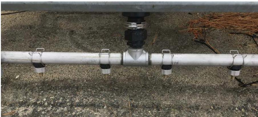
**Figure 13. Simple Spray Bank with Clip-On Nozzles (Caltrans / VariTech)**
