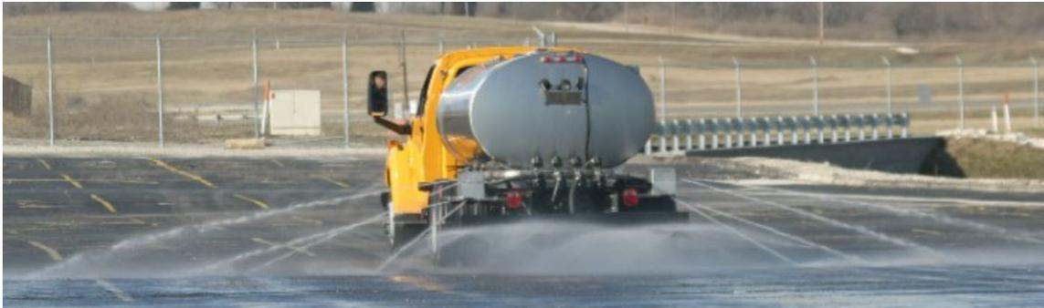
**Figure 18. Multi-Lane Brine Spraying**
