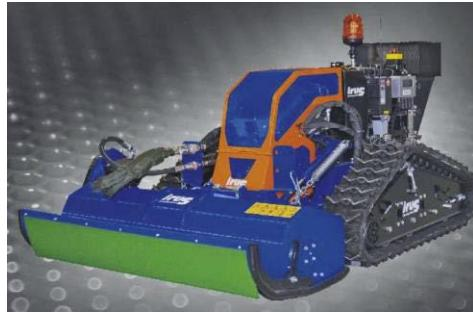
Figure 23. Deltrak 2.5 RC Tool-Carrier Tractor
