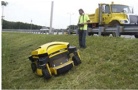
Figure 4. Illinois TA Operating ILD02 RC Mower
