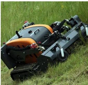
**Figure 20. RoboFlail plus RC Tool-Carrier Tractor**
