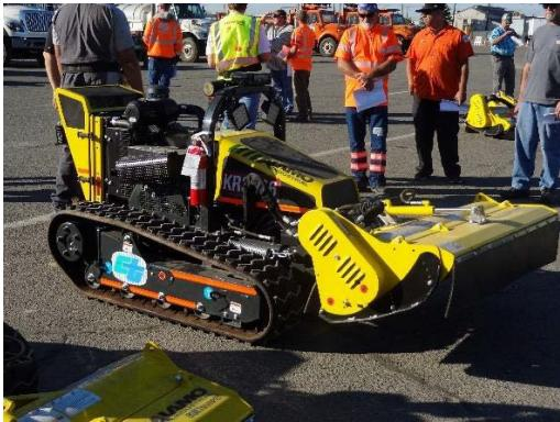
**Figure 14. Caltrans Traxx-RF RC Tool-Carrier Tractor**
