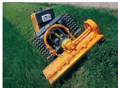
**Figure 21. RoboFlail vario RC Tool-Carrier Tractor**
