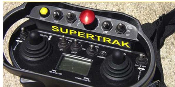
Figure 2. Wireless Controller with LCD display
