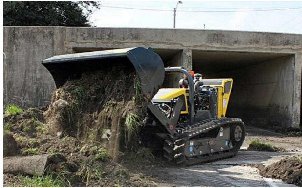
**Figure 15. RoboGreen RC Tool-Carrier Tractor Equipped with Bucket**
