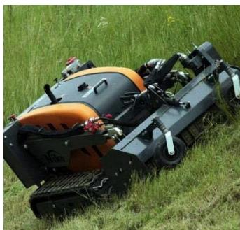
**Figure 20. RoboFlail plus RC Tool-Carrier Tractor**
