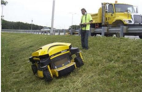
Figure 4. Illinois TA Operating ILD02 RC Mower
