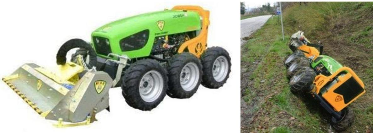
**Figure 21. Green Climber Power-6 RC Tool-Carrier Tractor**
