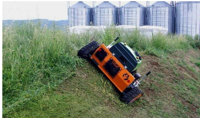
**Figure 11. Mini Green Climber RC Mower**
