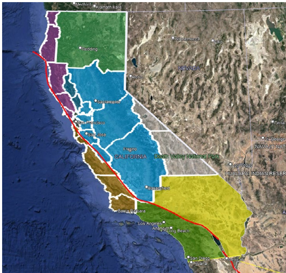
Map of Regional Boundaries for Sub-networks of the Caltrans Spatial Reference Network (CTSRN)
