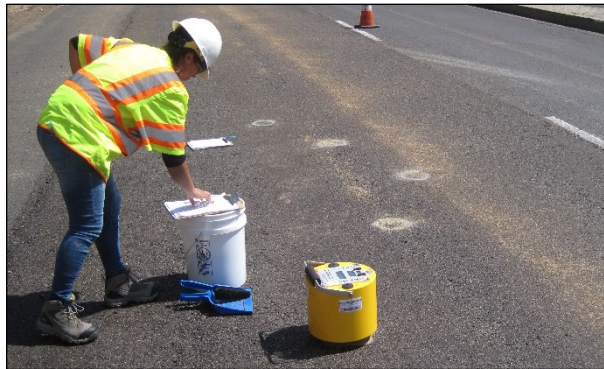
Figure 3.13: Soil stiffness gauge.
