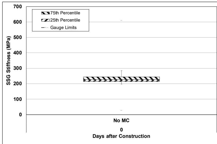
Figure B.193: Cell S25: SSG measured stiffness.
