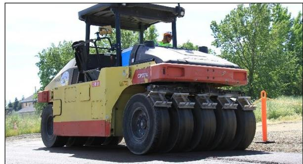
**Figure 6.14: Pneumatic-tired roller on a PDR layer.**
