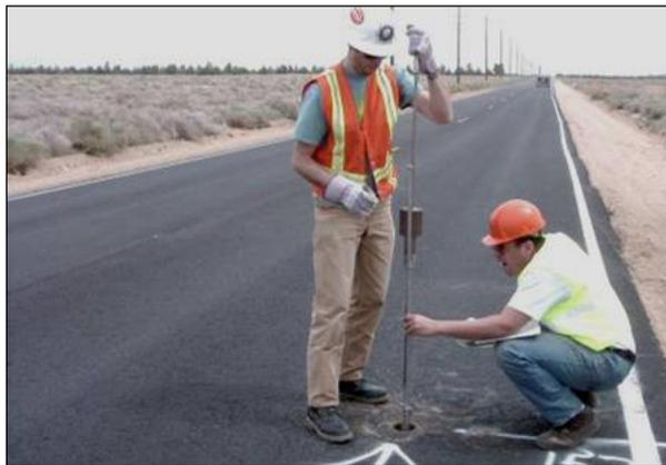
Figure 2.52: DCP test.
