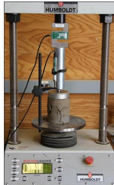
Figure 5.9: Unconfined compressive strength test.
