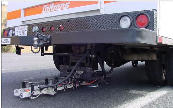
**Figure 2.53: Falling weight deflectometer, vehicle mounted.**
