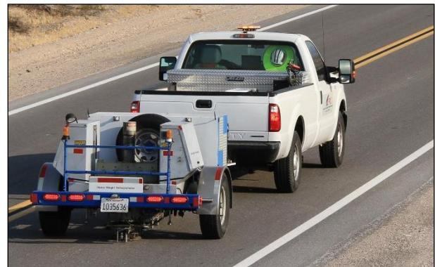
**Figure 2.54: Falling weight deflectometer, trailer mounted.**
