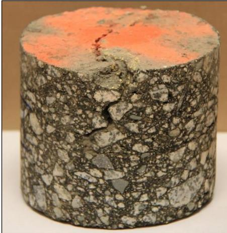
Figure 2.41: Top-down thermal crack.
