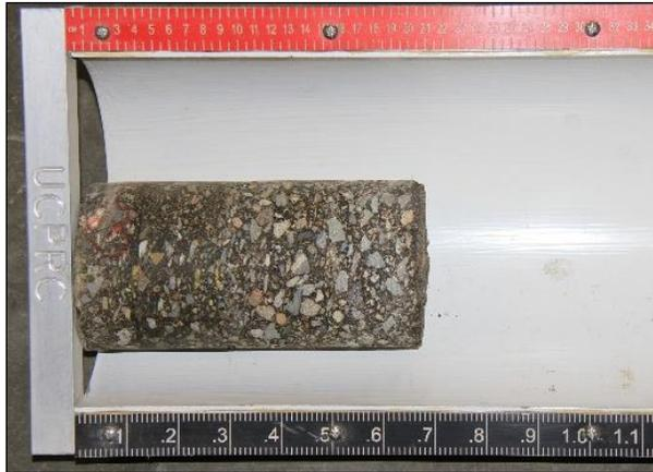
**Figure 2.40: Core measurement.**
