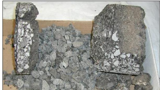
**Figure 2.48: Stripped asphalt concrete layer.**
