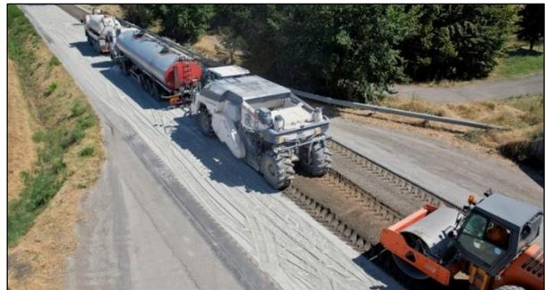
Figure 1.5: Full-depth recycling train (wheel).
