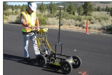
**Figure 2.55: Ground penetrating radar systems.**
