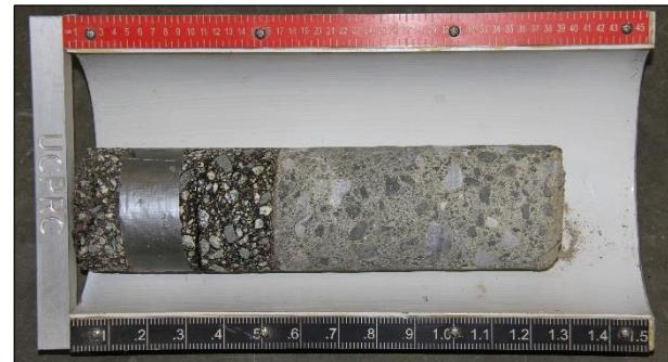
Figure 2.44: Asphalt on cement-treated base.
