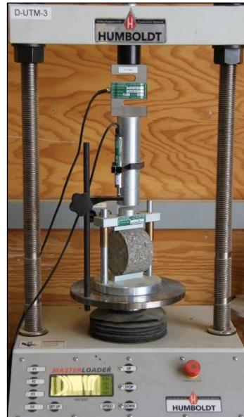
Figure 5.3: Indirect Tensile Strength Test.
