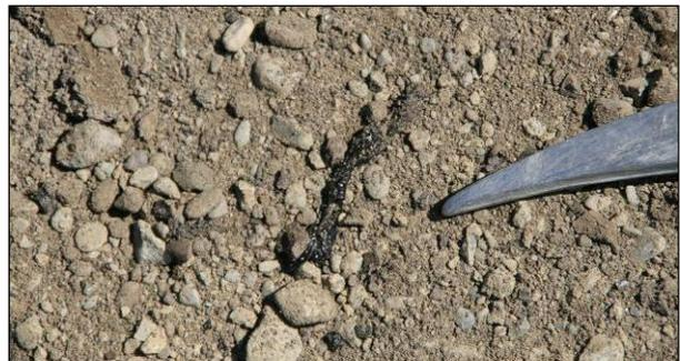
Figure 6.42: Unfoamed binder in recycled material on an FDR-FA project.
