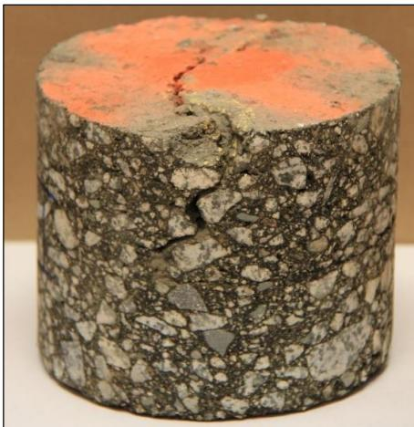
Figure 2.41: Top-down thermal crack.
