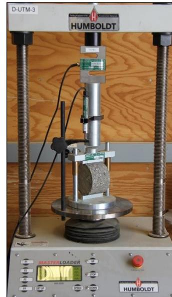
**Figure 5.3: Indirect Tensile Strength Test.**
