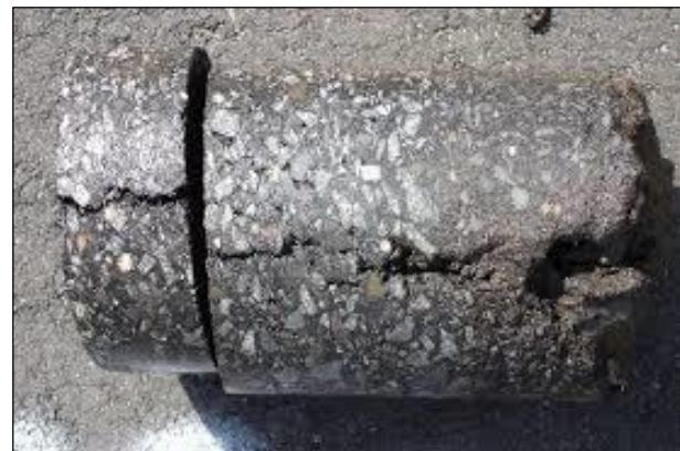
Figure 2.42: Bottom-up fatigue/reflected crack.
