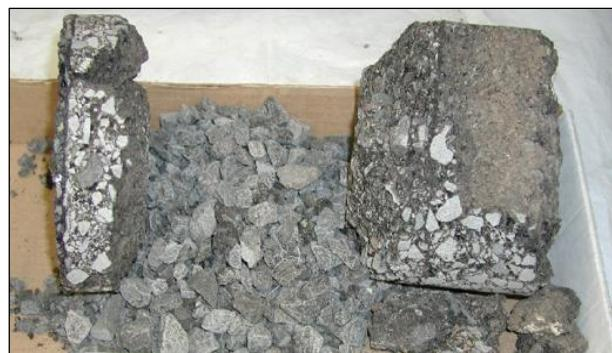
**Figure 2.48: Stripped asphalt concrete layer.**
