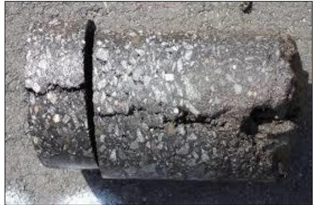
Figure 2.42: Bottom-up fatigue/reflected crack.
