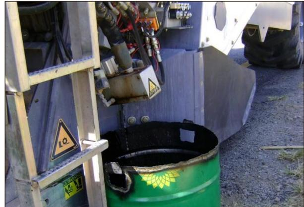
**Figure 6.26: Nozzle for checking binder foaming characteristics.**
