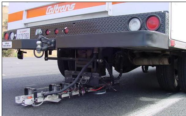
**Figure 2.53: Falling weight deflectometer, vehicle mounted.**
