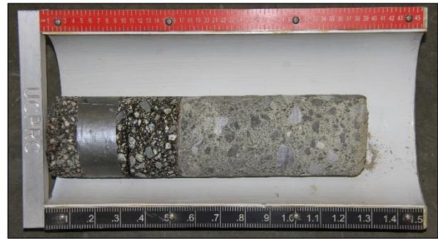
Figure 2.44: Asphalt on cement-treated base.
