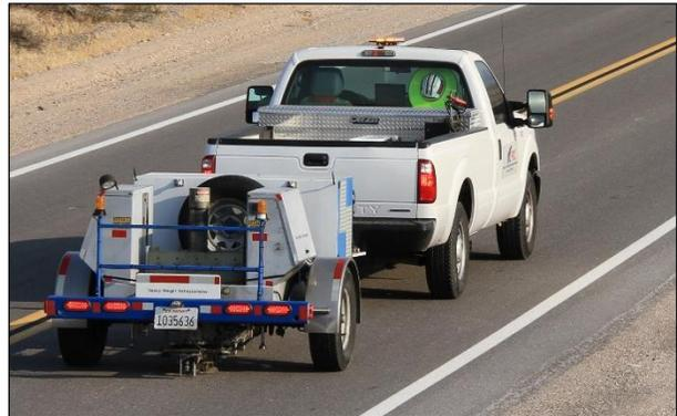
**Figure 2.54: Falling weight deflectometer, trailer mounted.**
