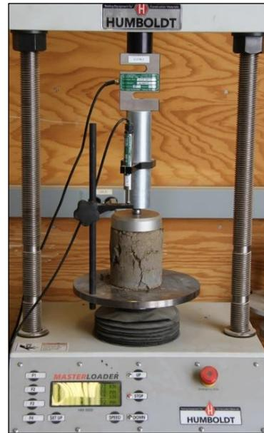
**Figure 5.9: Unconfined compressive strength test.**
