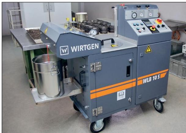
Figure 5.4: Laboratory foaming equipment.
