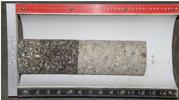
Figure 2.43: Concrete beneath asphalt layers (composite pavement).
