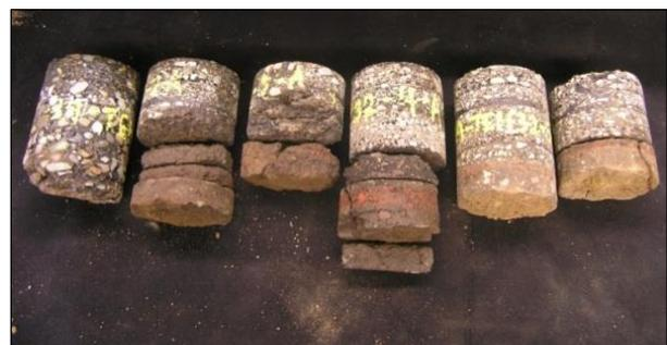
**Figure 2.50: Degrees of adhesion of asphalt concrete layer to unbound base.**
