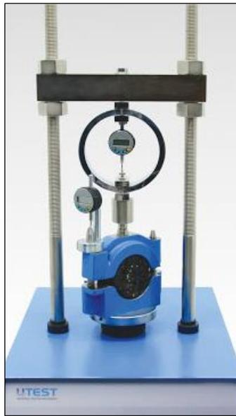
**Figure 5.2: Marshall Stability Test.**
