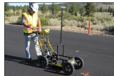
**Figure 2.55: Ground penetrating radar systems.**
