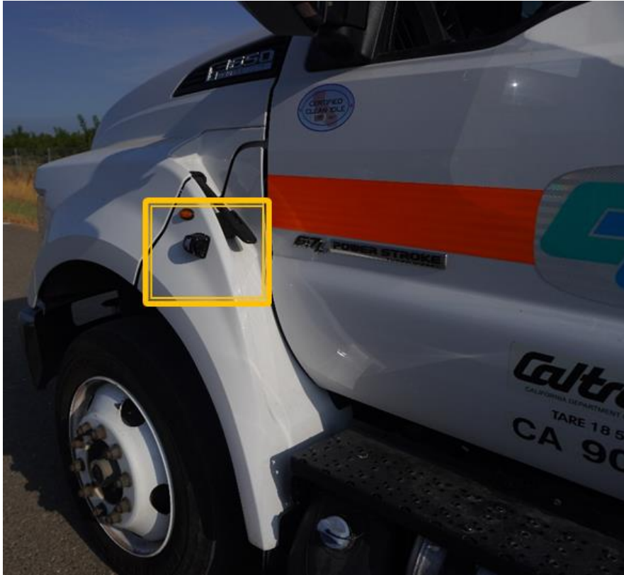
Figure 2.5: Location of left rear facing camera on the TMA truck
