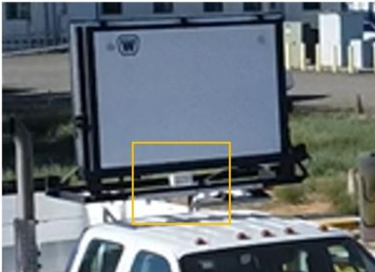
Figure 2.8: iCone mounting location on a truck with a changeable message sign
