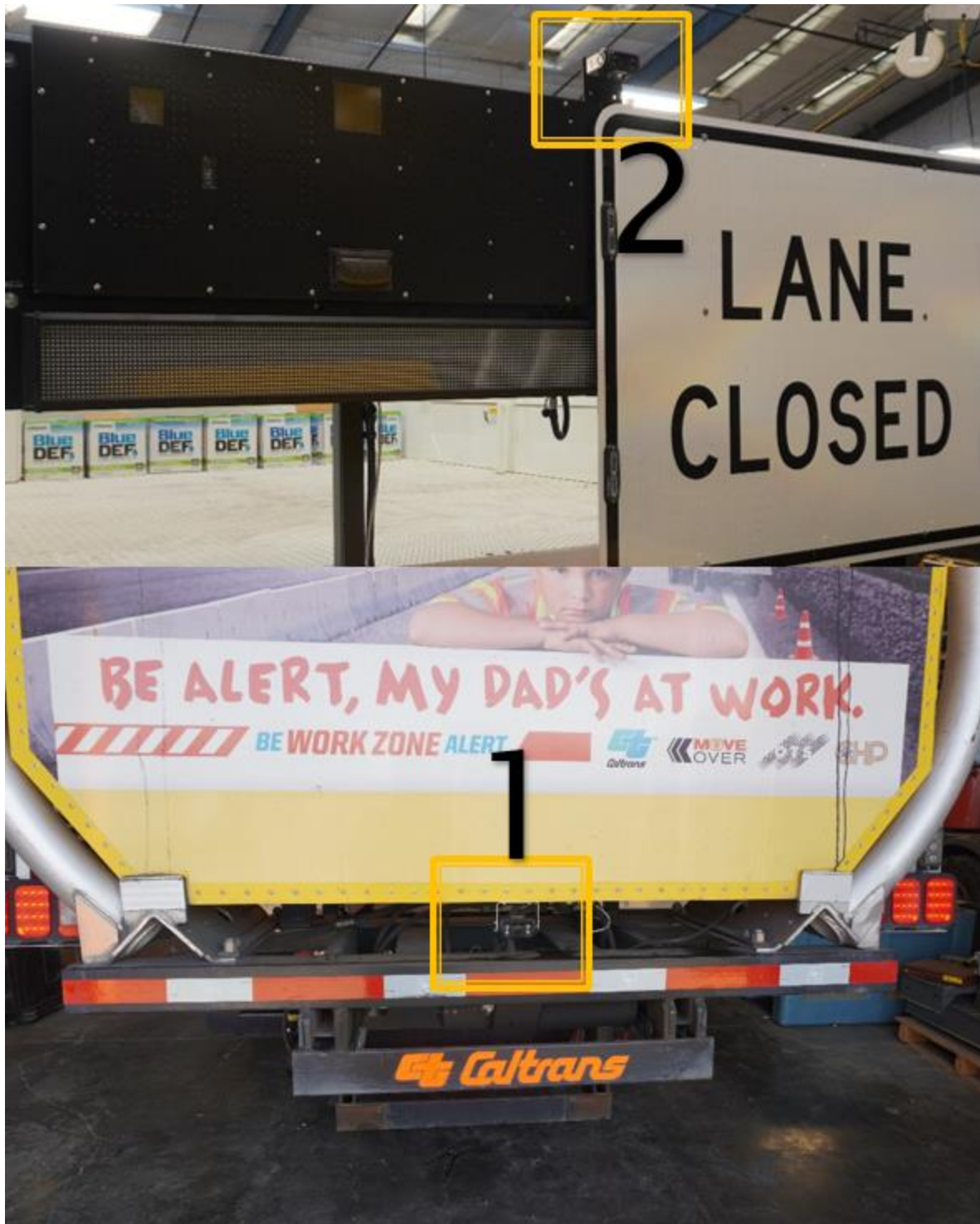
Figure 2.4: Location of rear facing cameras on the TMA truck
