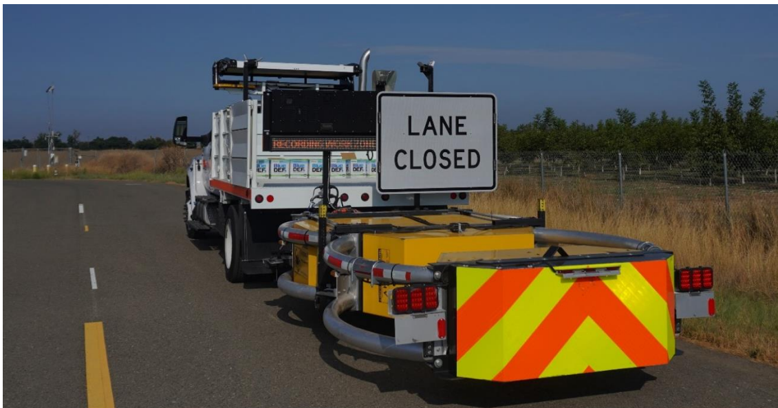
Figure 2.3: Kohltech radar signboard and mini-messenger sign next to LANE CLOSED sign
