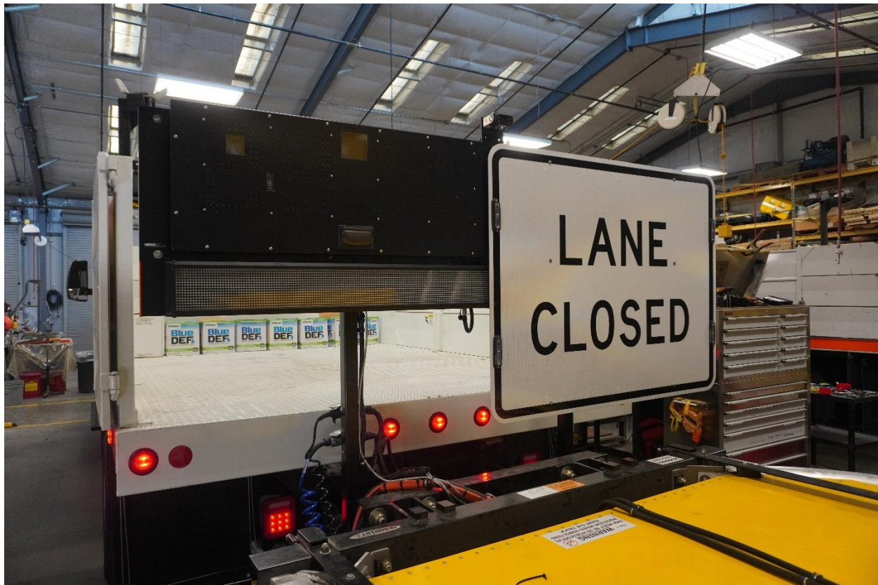
Figure 2.13: Radar signboard and LANE CLOSED sign installed on a TMA truck
