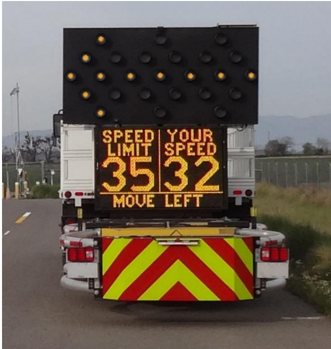
Figure 2.2: TrafficCalm radar signboard evaluated in the previous research task 3685
