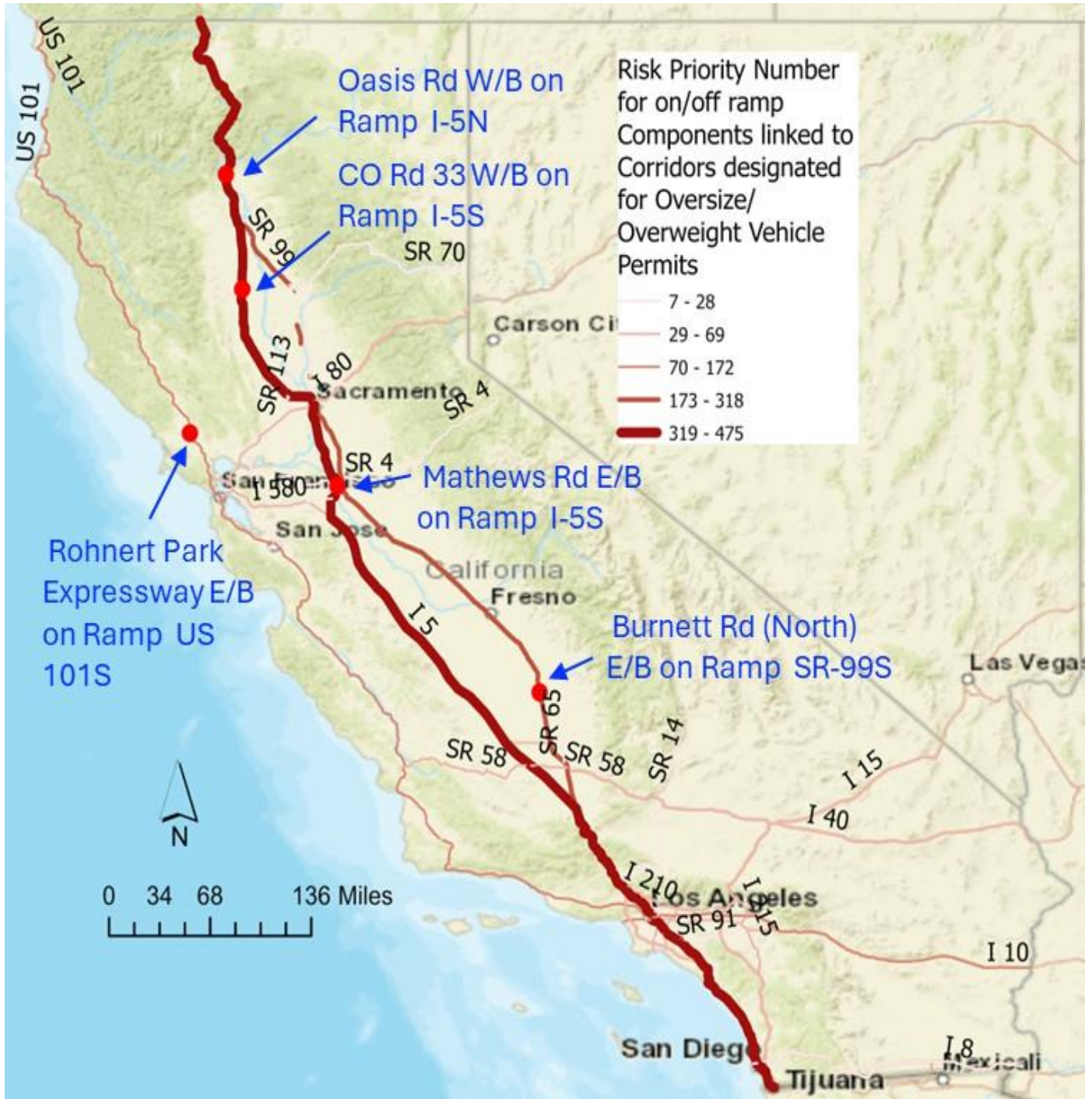
Figure 16: Spatial distribution of Risk Priority Numbers for on/off ramp components linked to corridors designated for oversized/overweight vehicle permits
