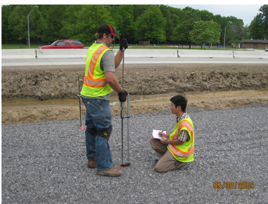
Dynamic cone penetrometer testing on open graded drainage course layer on I 94 project in Michigan (May 30, 2009)
