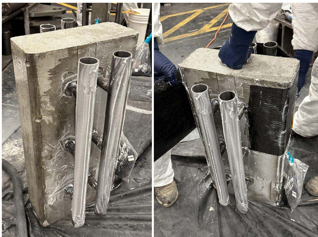
Figure 18 Wrapping of FRP sheets on the steel tubes and concrete.
