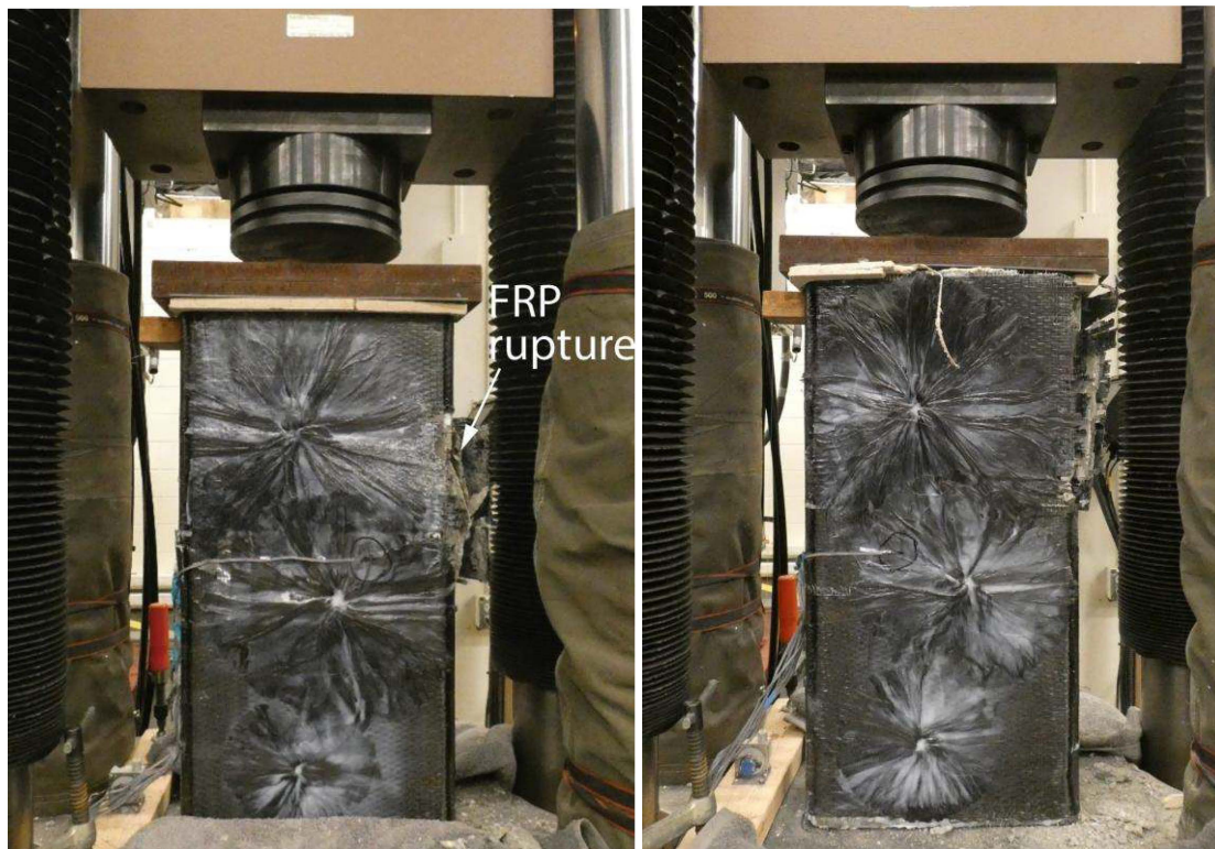
Figure 30 Failure mode of Group 3 columns.
