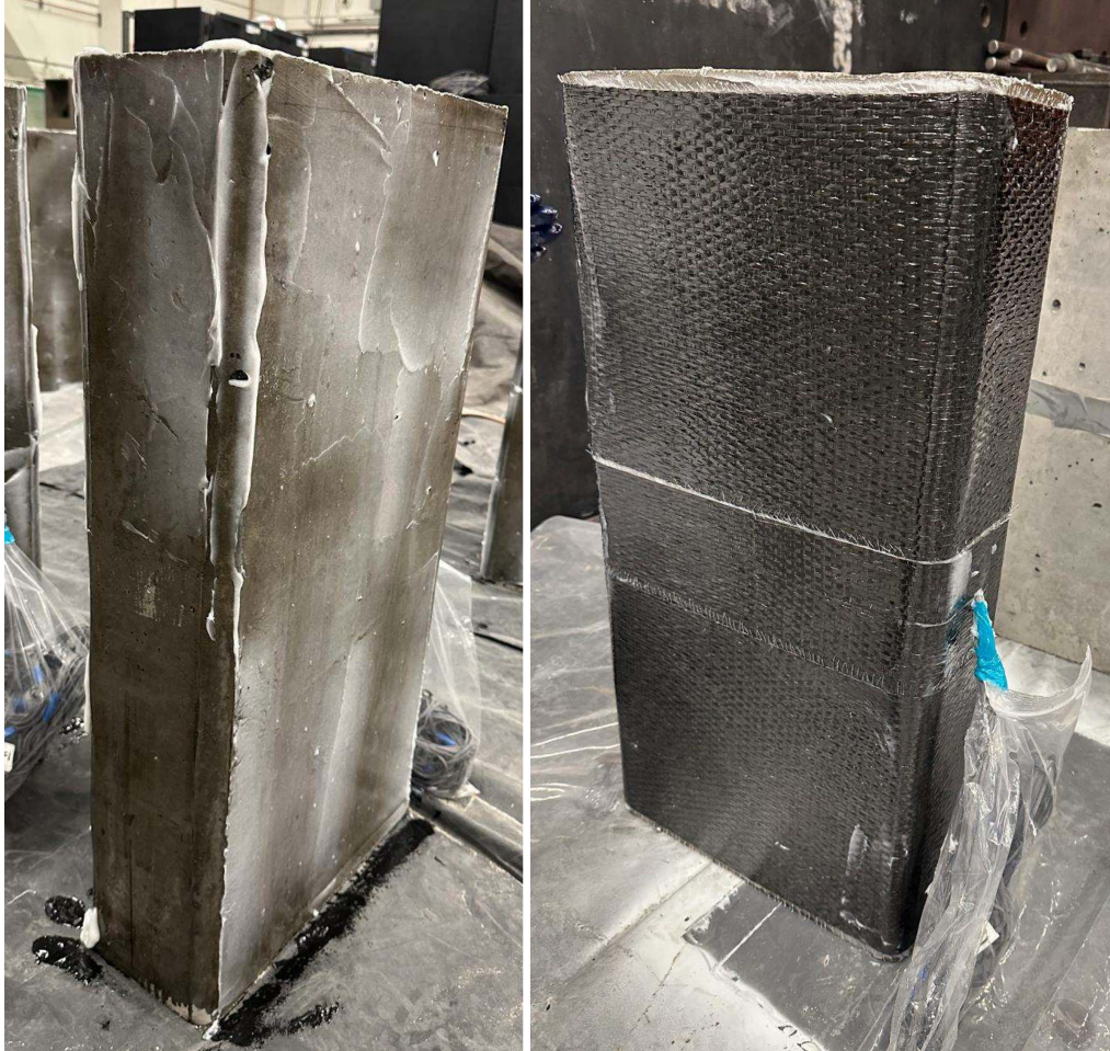
Figure 10 Priming and wet layup of FRP jacketed columns with no anchors.
