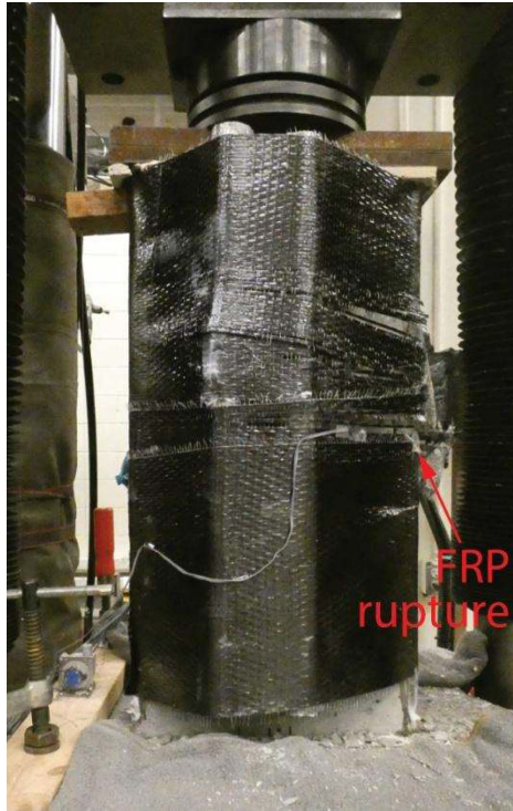
Figure 45 Failure mode of Group 6 Column 1.
