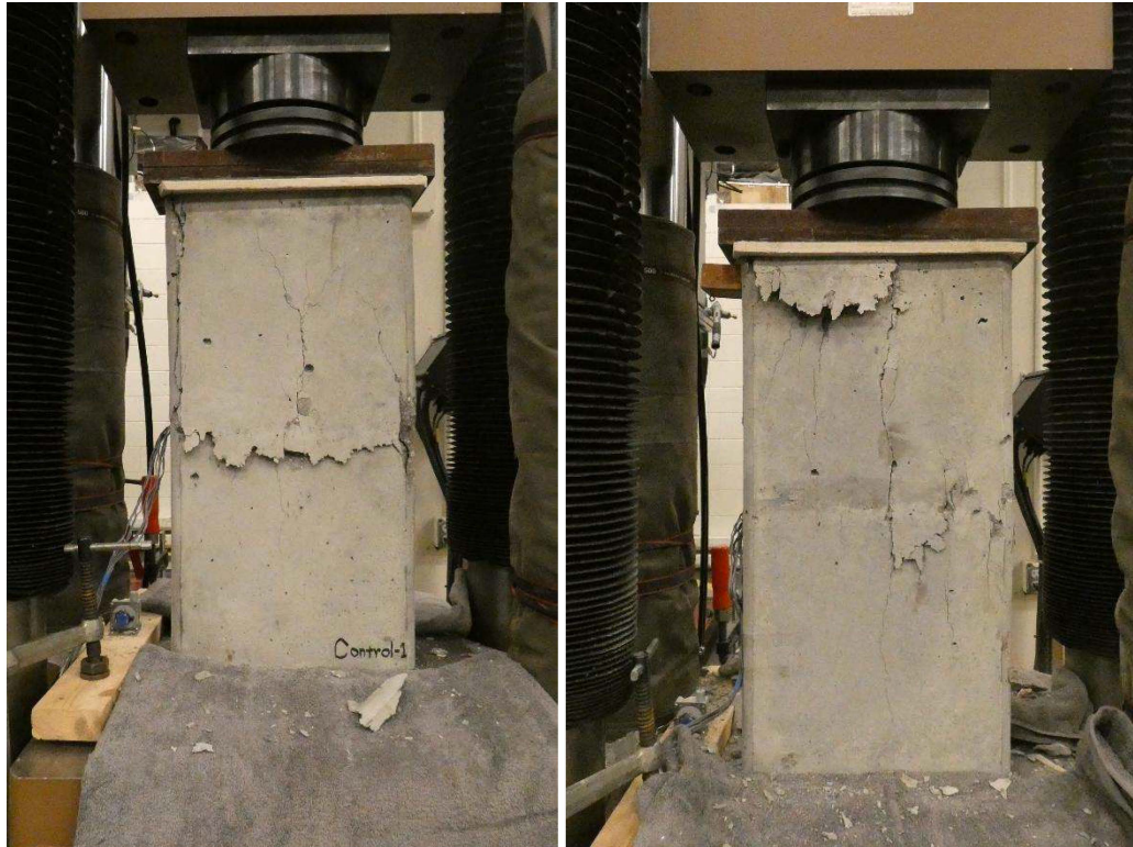
Figure 21 Failure mode of control columns.
