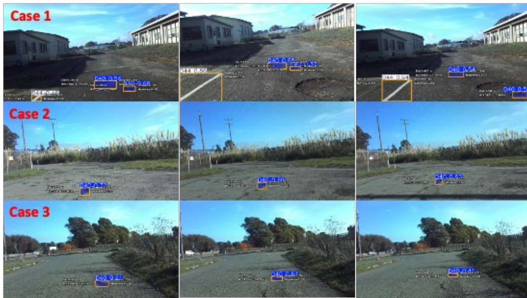
Figure 16. Pothole Size Estimation with Different Distances
