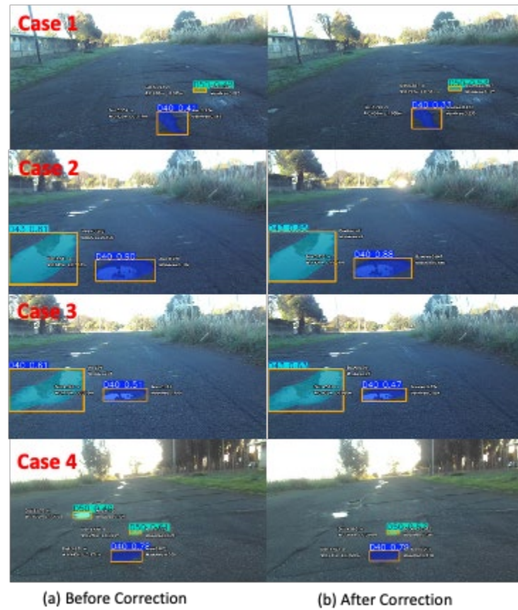
Figure 15. Pothole Size Estimation Before and After Correction
