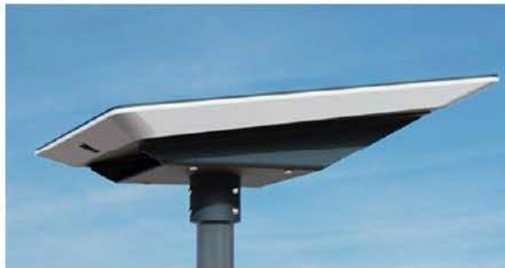
Figure A.11: Starlink Flat HP Pipe Adapter attached to the Wedge Mount Kit, which is in part screwed to the bottom of the antenna
