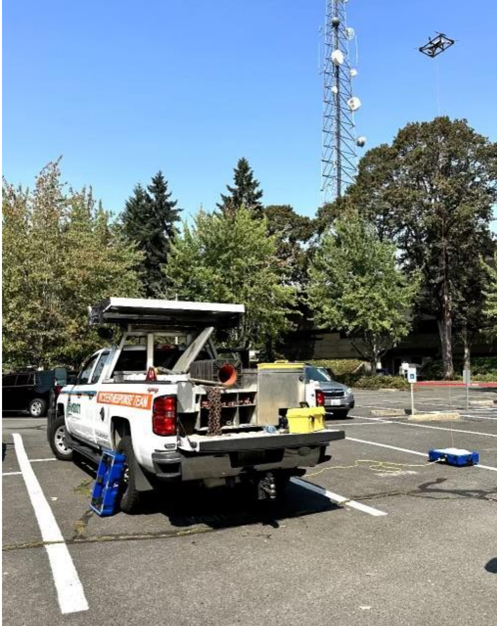
Figure 2.16: Fotokite cradle powered by a WSDOT vehicle. Photo courtesy of WSDOT
