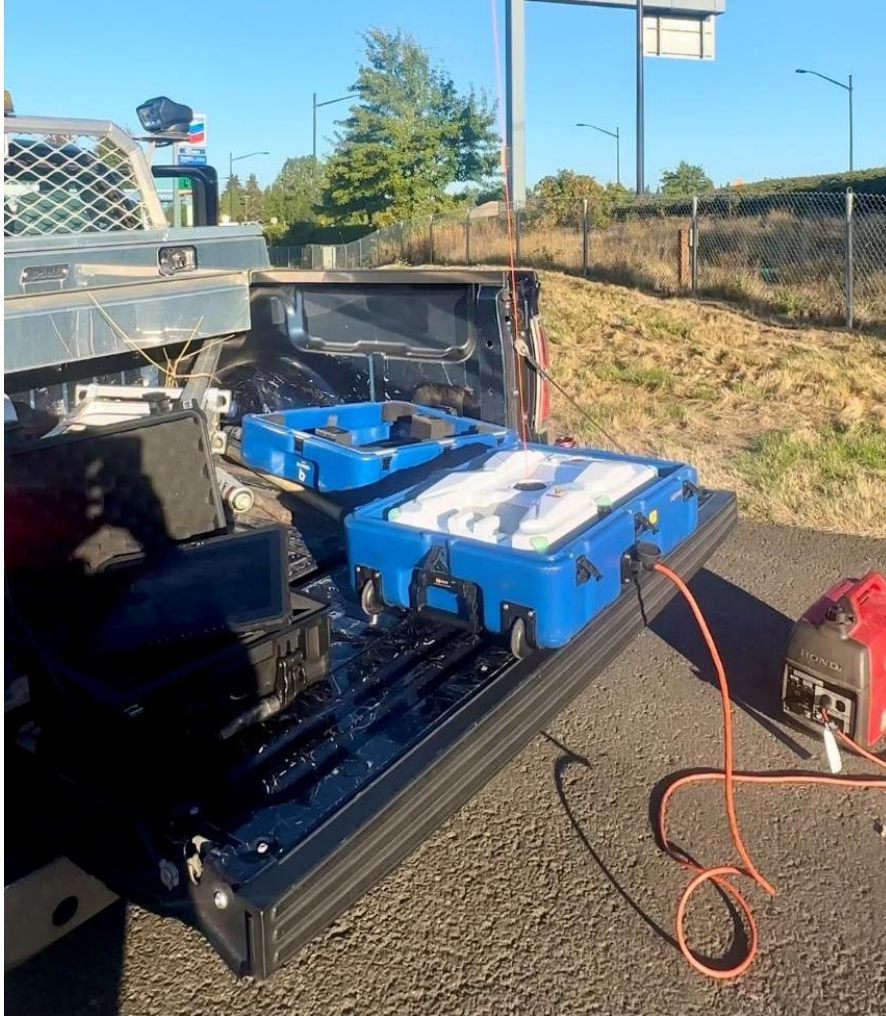
Figure 2.14: Fotokite powered by a Honda generator. Note that the cable shown in the photo was not provided by Fotokite; WSDOT used an alternative cable due to a malfunction with the original. Photo courtesy of WSDOT
