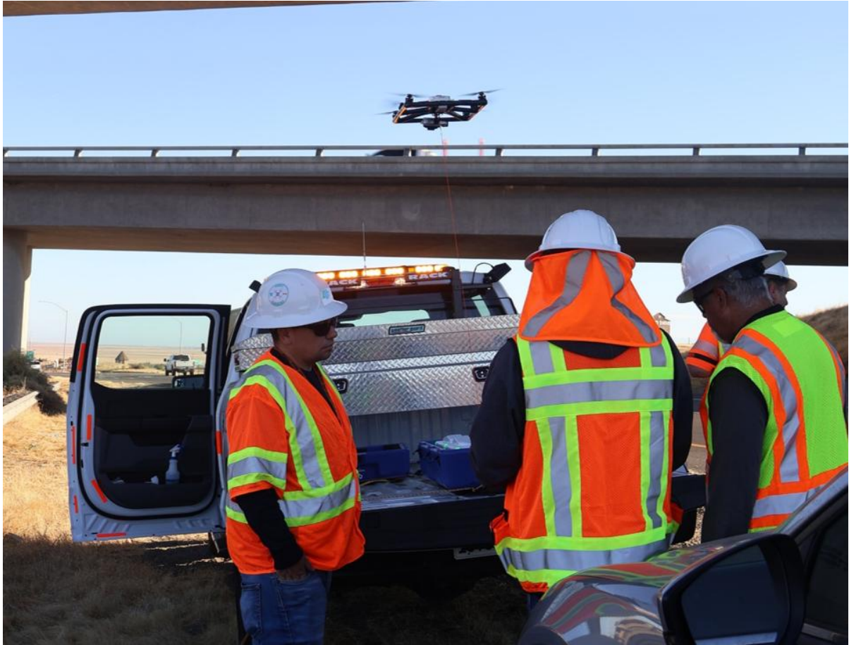
Figure 3.10: Example of the Fotokite deployment in a scheduled event. Footage was relayed back to the Caltrans TMC. Photo courtesy of Caltrans
