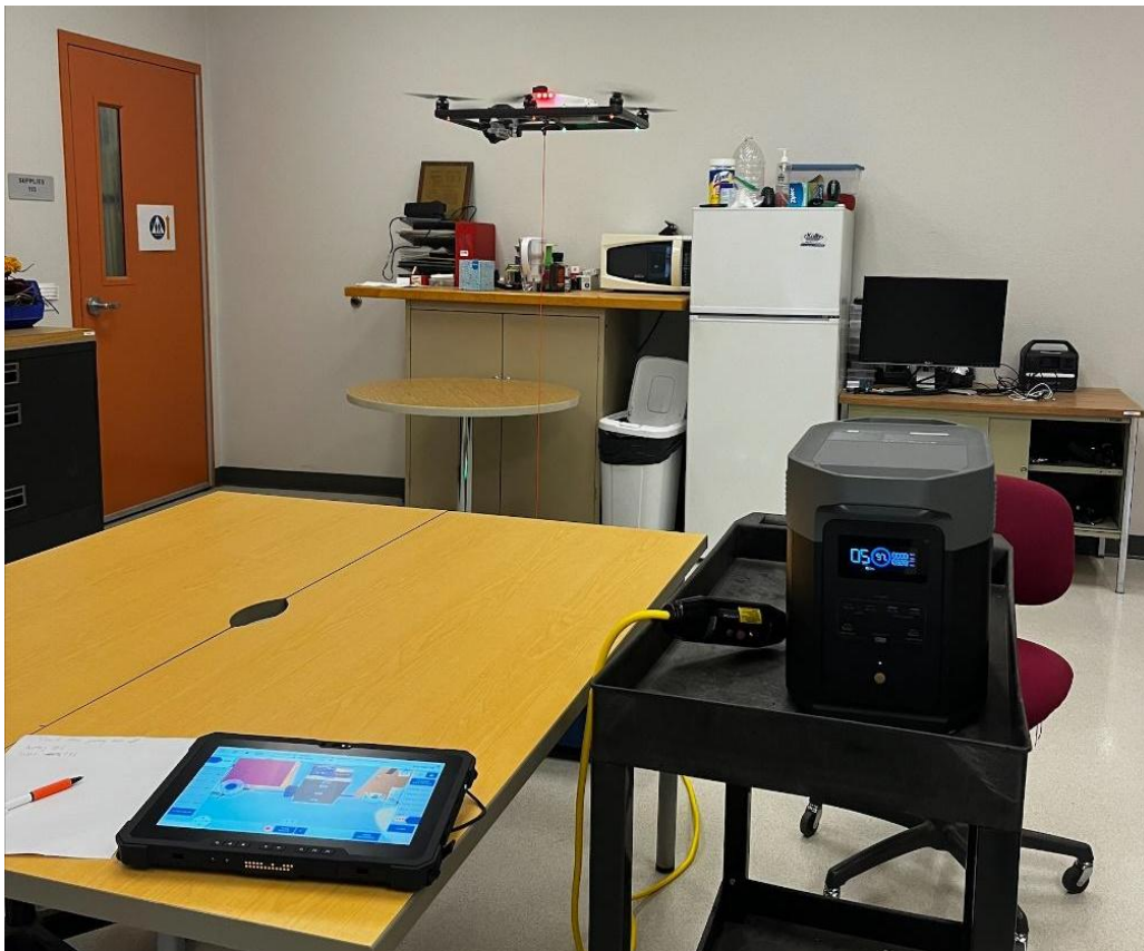
Figure 2.13: Fotokite powered by EcoFlow portable power station
