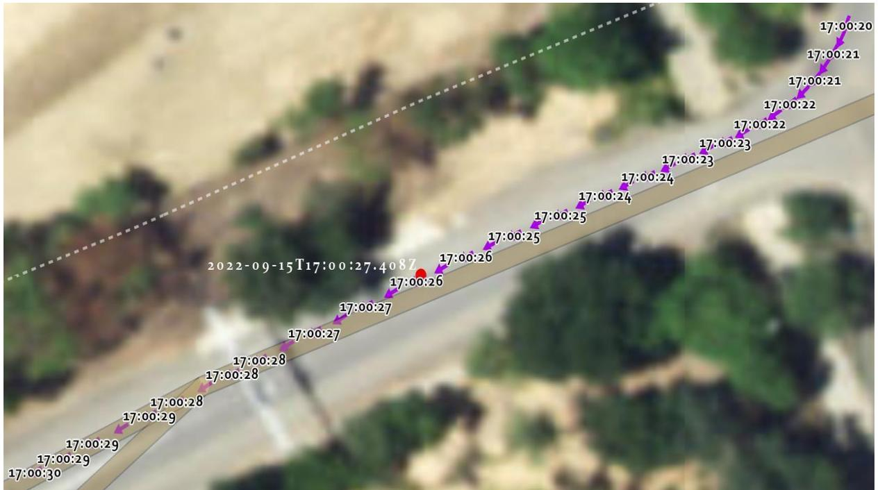
**Figure 4.6: Ramp 1 Trial 6 driving path (purple arrows) and received Bosch alert (red dot)**
