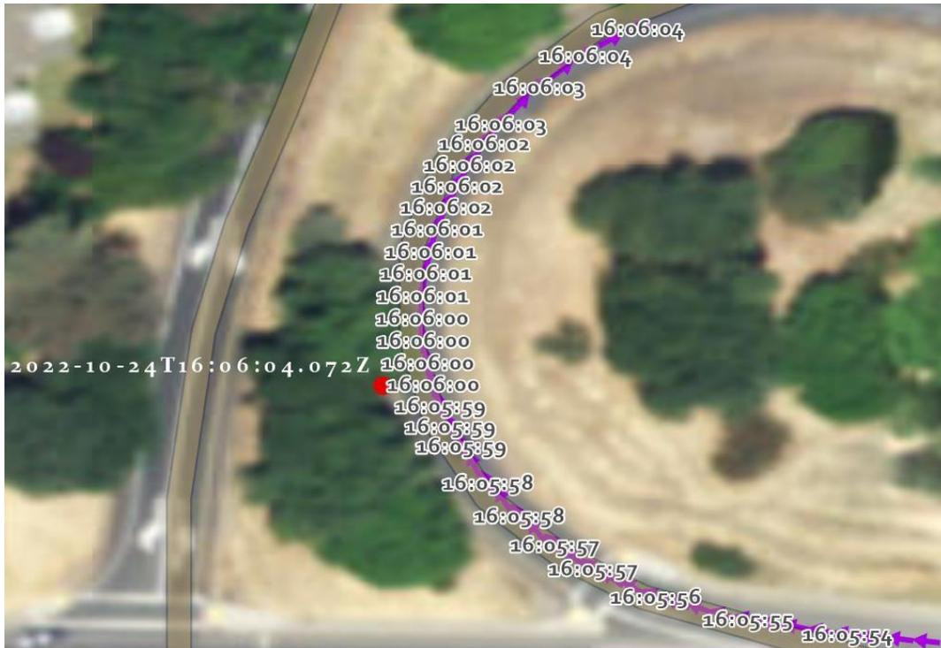
Figure 4.19: Ramp 2 Trial 8 driving path (purple arrows) and received Bosch alert (red dot)
