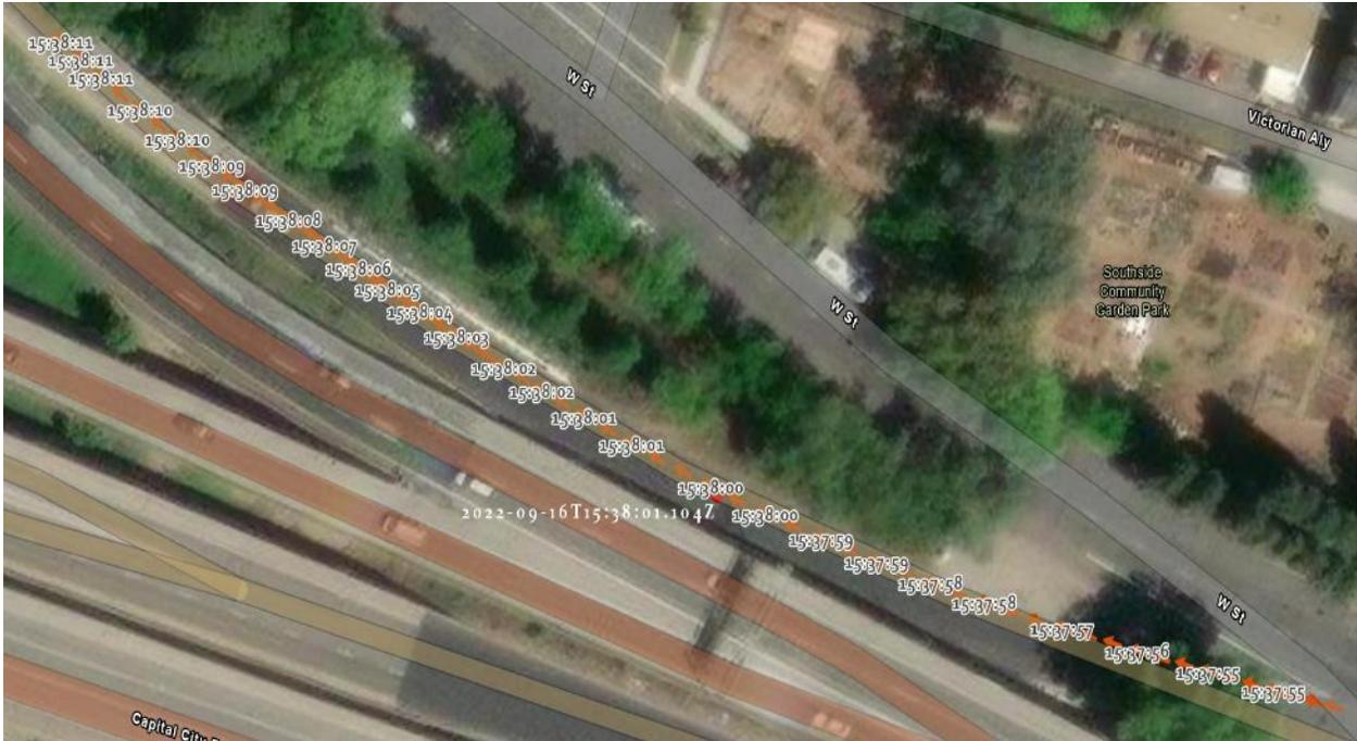
**Figure 4.27: Ramp 3 Trial 5 driving path (orange arrows) and received Bosch alert (red dot)**
