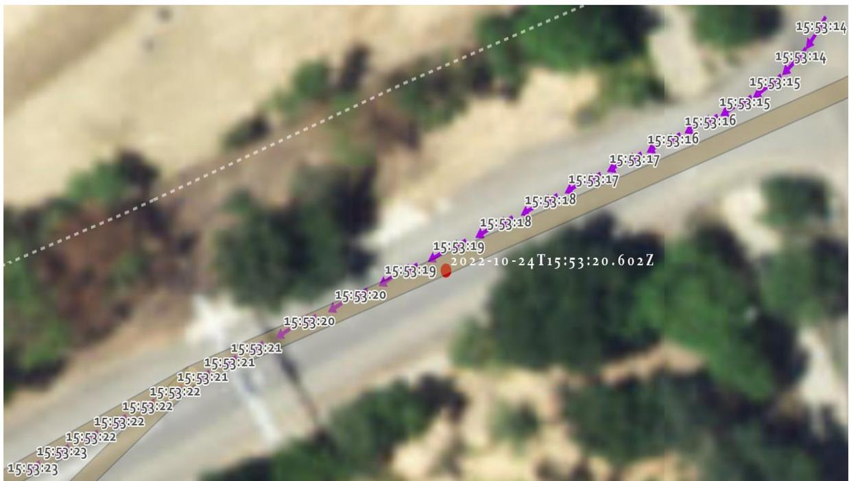
**Figure 4.7: Ramp 1 Trial 7 driving path (purple arrows) and received Bosch alert (red dot)**
