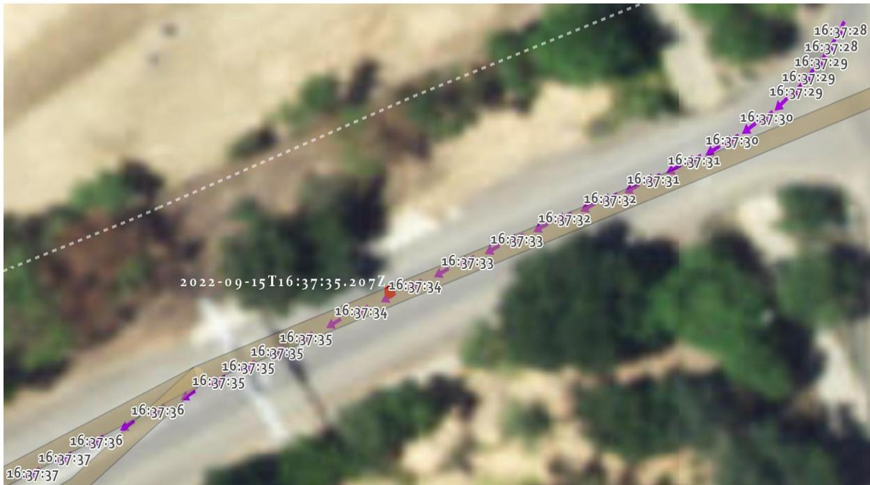
**Figure 4.4: Ramp 1 Trial 4 driving path (purple arrows) and received Bosch alert (red dot)**
