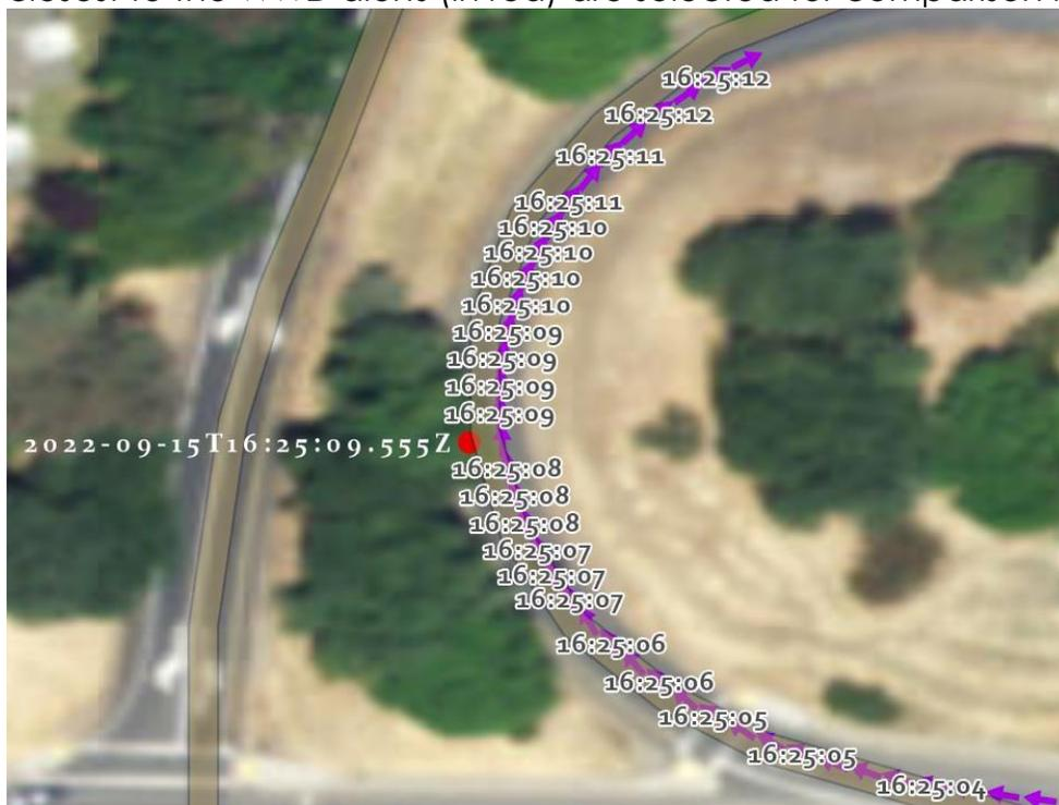
Figure 4.12: Ramp 2 Trial 1 driving path (purple arrows) and received Bosch alert (red dot)
