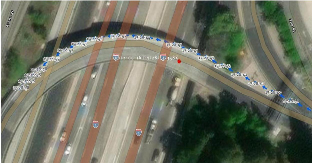
Figure 4.49: Ramp 5 Trial 5 driving path (blue arrows) and received Bosch alert (red dot)
