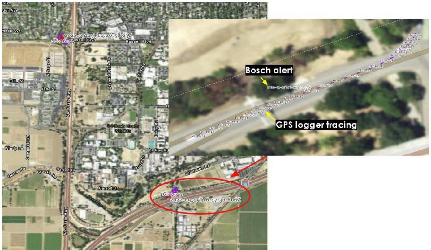
**Figure 3.17: Sample GPS logger results compared to WDW alerts on ArcGIS Pro**
