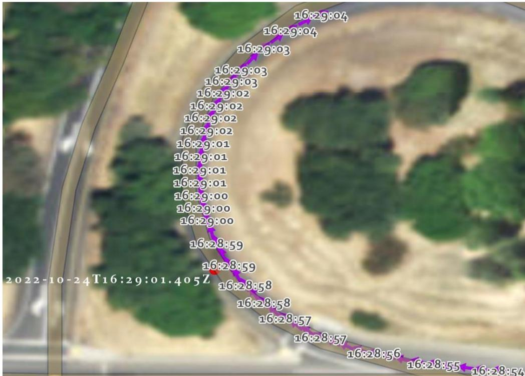
Figure 4.21: Ramp 2 Trial 10 driving path (purple arrows) and received Bosch alert (red dot)
