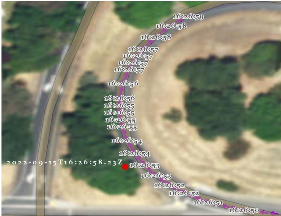
Figure 4.13: Ramp 2 Trial 2 driving path (purple arrows) and received Bosch alert (red dot)
