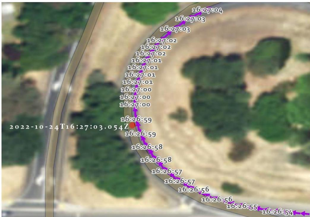
Figure 4.18: Ramp 2 Trial 7 driving path (purple arrows) and received Bosch alert (red dot)
