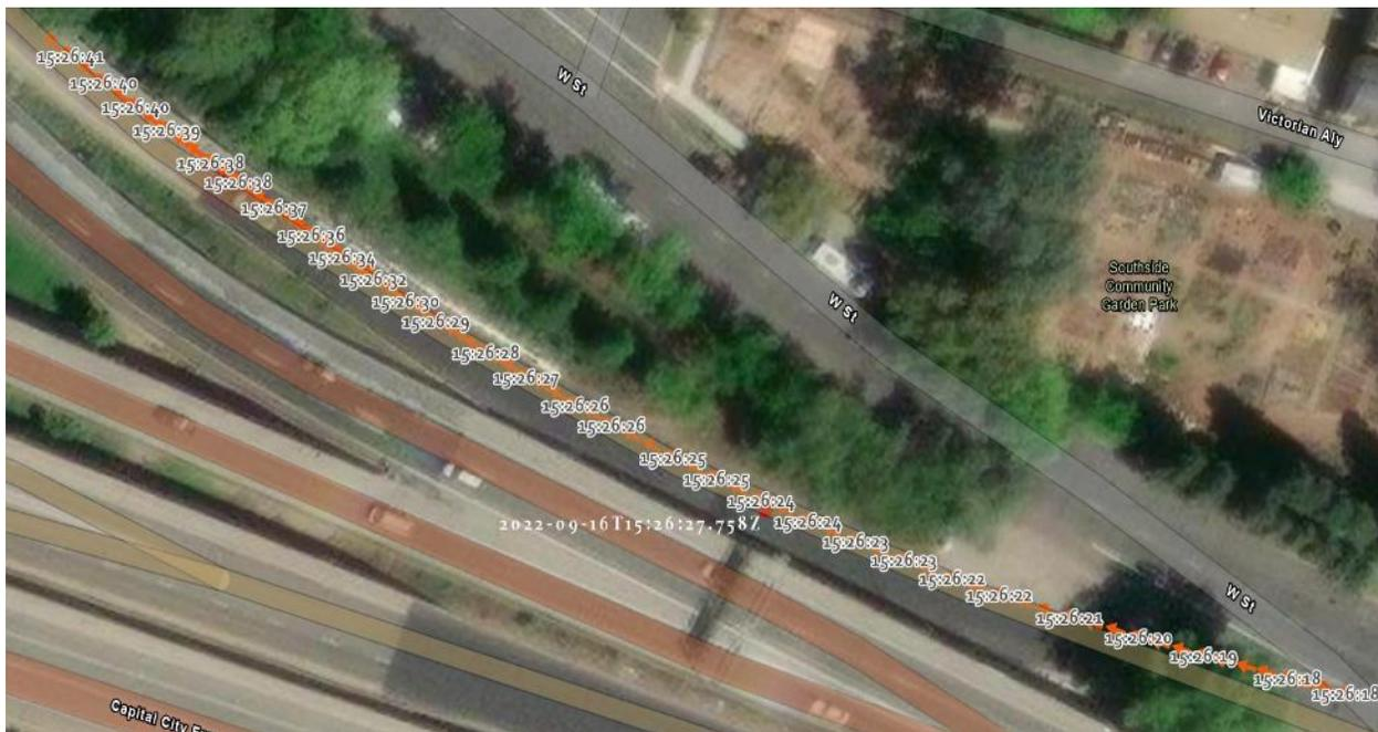
**Figure 4.26: Ramp 3 Trial 4 driving path (orange arrows) and received Bosch alert (red dot)**
