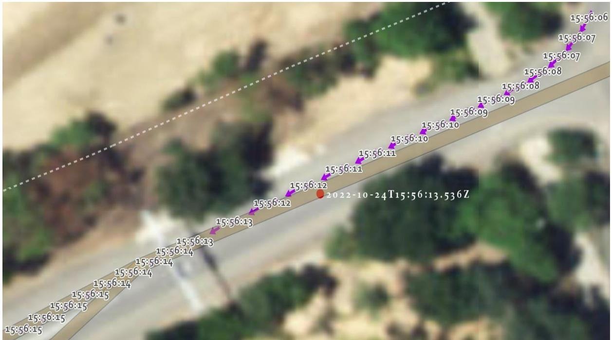
**Figure 4.8: Ramp 1 Trial 8 driving path (purple arrows) and received Bosch alert (red dot)**
