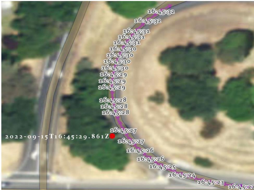
Figure 4.15: Ramp 2 Trial 4 driving path (purple arrows) and received Bosch alert (red dot)
