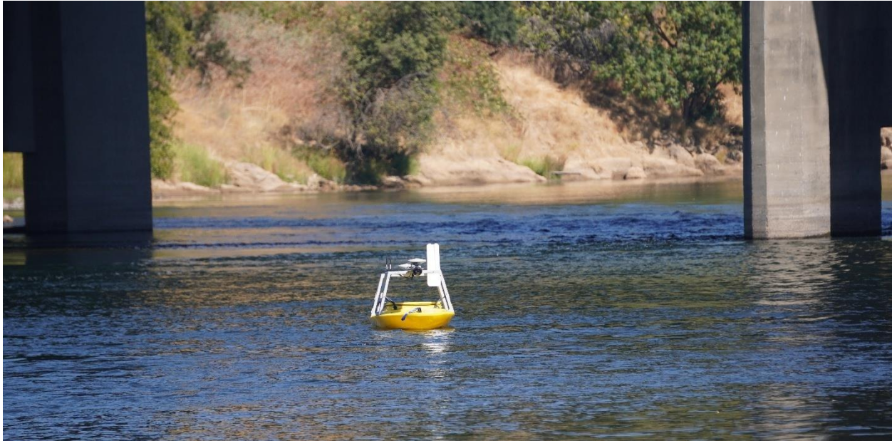
Figure 3.6: EchoBoat-160 bathymetric survey platform pilot project at Sunrise Boulevard over American River in Sacramento
