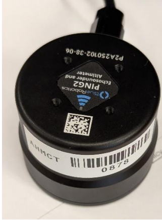
Figure 4.3: Blue Robotics Ping 2 Sonar for underwater obstacles detection
