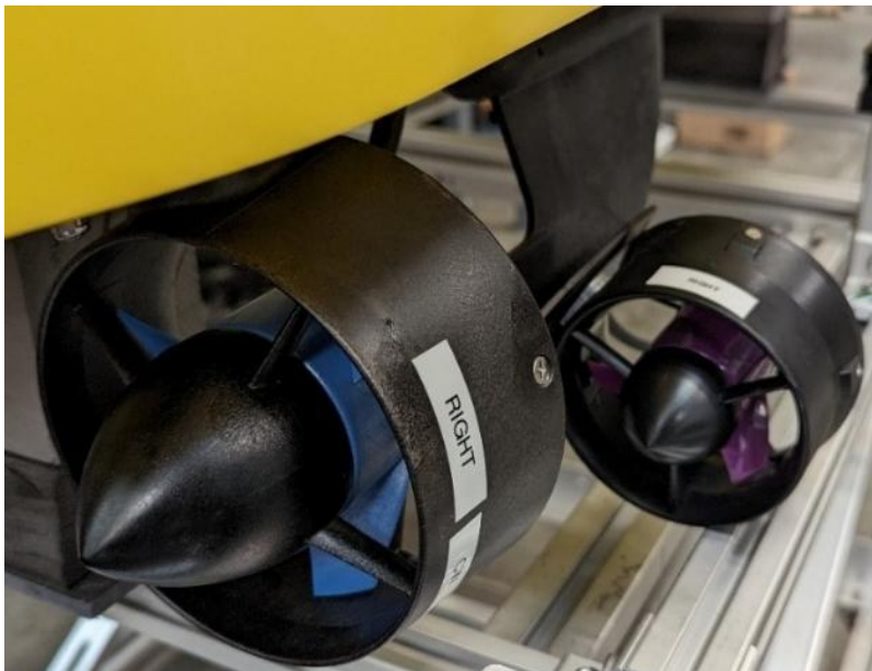
Figure 2.4: Size comparison between original EchoBoat-160 thruster (purple propeller blade) and the T-500 thruster (blue propeller blade)
