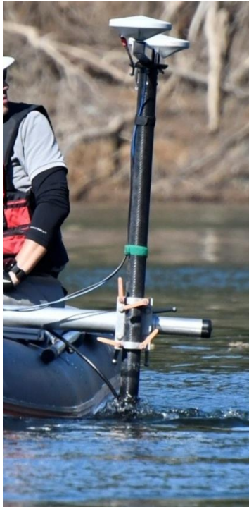
Figure 5.2: GNSS antennas and MBES sensor assembly flipped down with the MBES sensor below water
