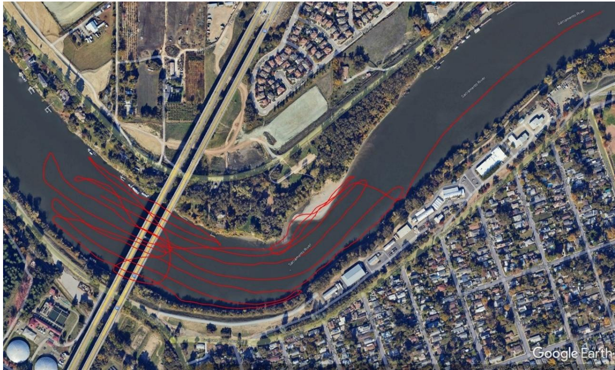
Figure 5.5: Caltrans inflatable boat survey path on Sacramento River near I-80 highway at Sacramento. Image courtesy of Google Earth.
