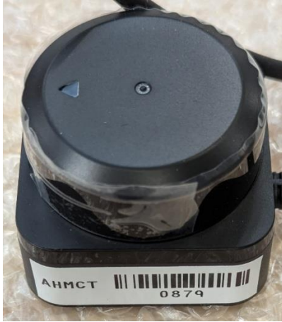
Figure 4.2: Slamtec S3 LiDAR 360-degree LiDAR for above water obstacles detection
