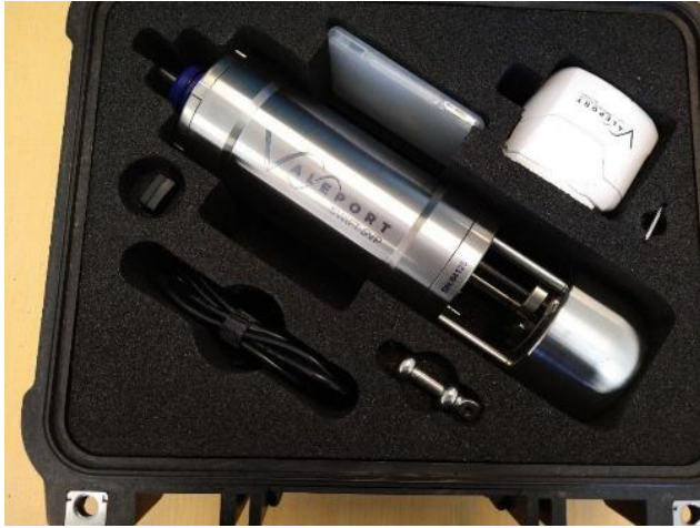
Figure 1.1: Valeport SWiFT Sound Velocity Profiler data logger for measuring water sound velocity, water temperature, and pressure at different water depths
