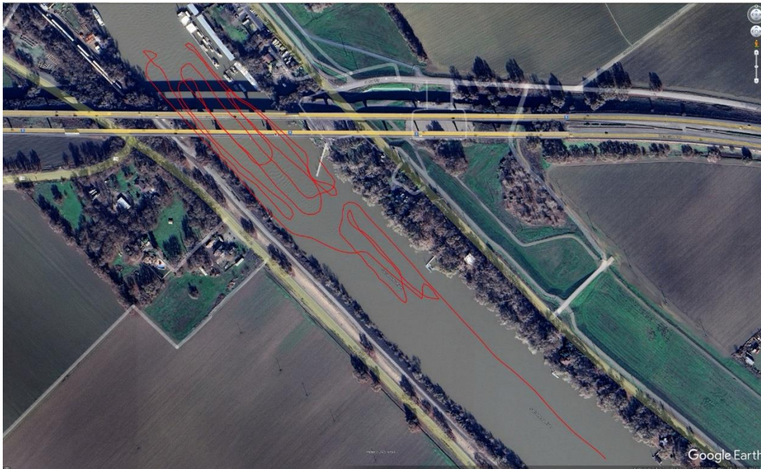
Figure 5.7: Caltrans inflatable boat survey path on Sacramento River near interstate highway 5 at Sacramento Airport. Image courtesy of Google Earth.
