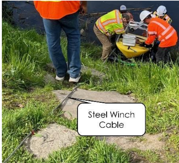
Figure 3.11: EchoBoat-160 launching from riverbank using custom cart attached to a vehicle winch line to control the descent into the water. Image courtesy of Caltrans.
