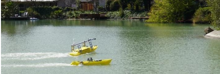
Figure 3.2: EchoBoat-160 and research USV testing at Stonegate Lake in Davis, California. EchoBoat-160
