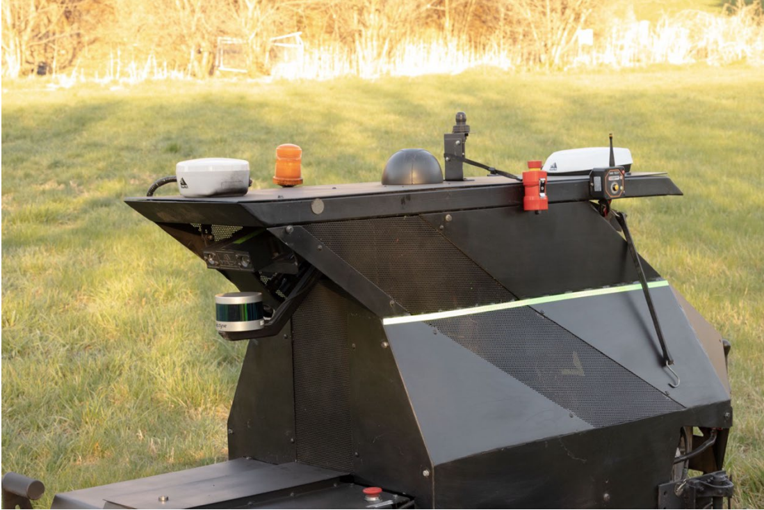
Figure 6.5. Top view of mower showing LIDAR, GPS, and power controls
