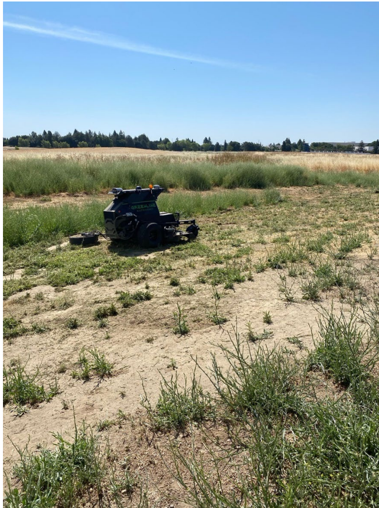
Figure 6.9. Greenline Autonomous Mower operating on level terrain
