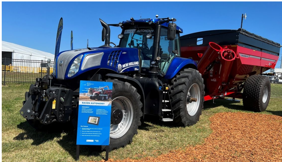
Figure 6.2. New Holland/Case IH Autonomous Tractor: Front and side view showing the guidance systems
