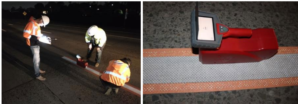
Figure 4.2: Left: Striping quality measurements performed by AHMCT researcher and Caltrans staff days after orange striping installation. Right: Retroreflectivity and nighttime color measurements on tape striping on I-5 NB south of Las Flores Overcrossing
