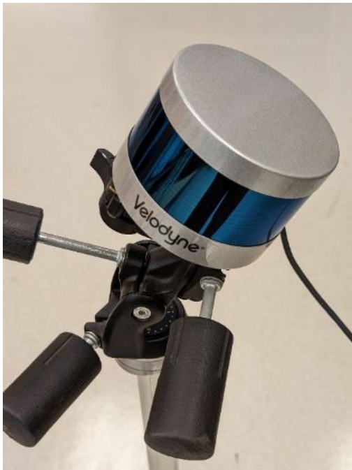
Figure A2.1: Velodyne VLP16 LiDAR sensor with a 30 degree tilt from the horizon
