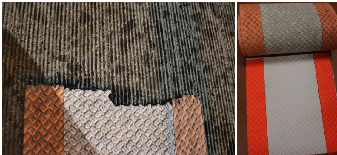
Figure 4.17: Left: Tape on freeway concrete surface with grinding grooves and orange tape striping worn (at 5 months). Right: New orange striping tape
