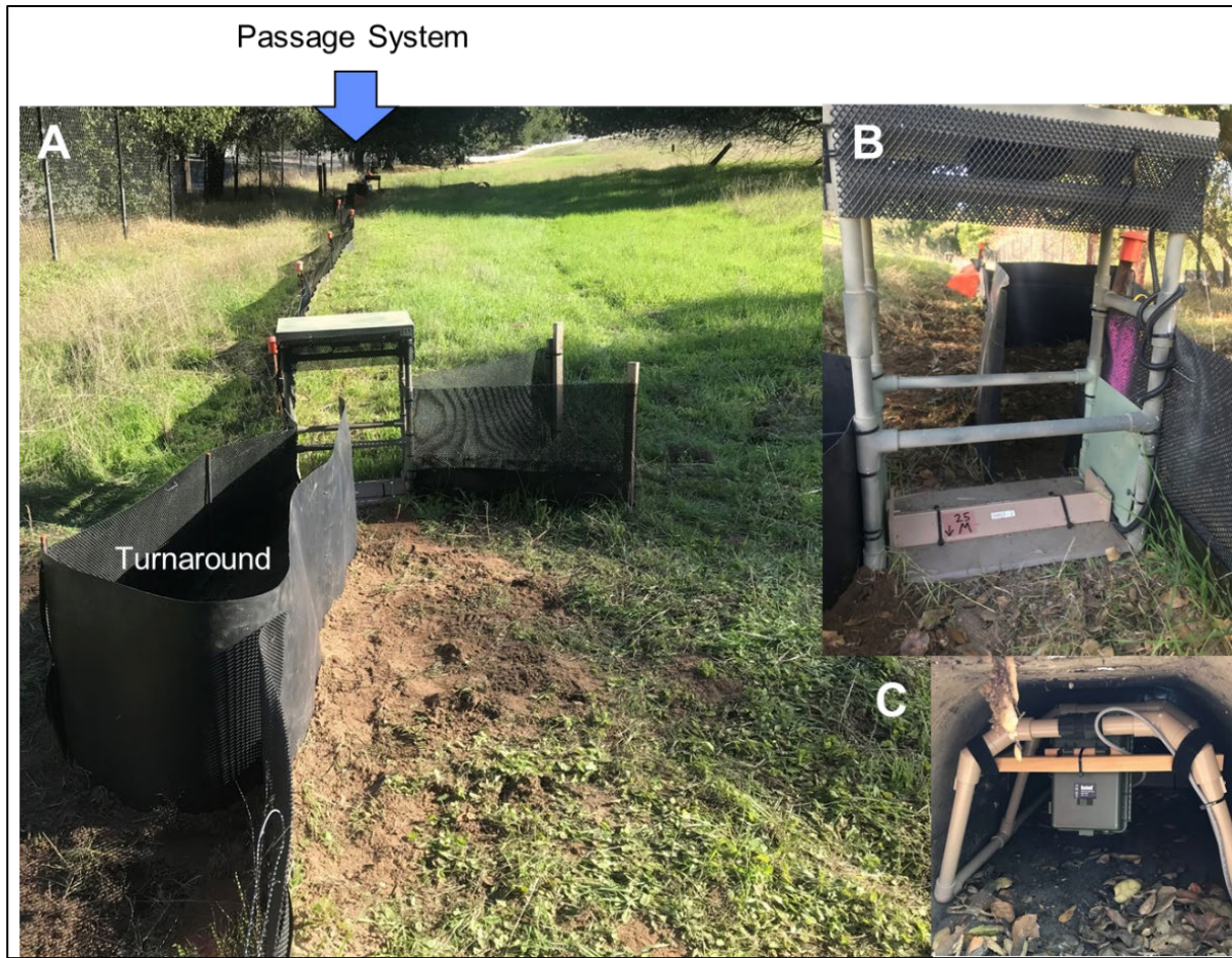
Figure2. Photo of turnaround along fence line (A), HALT camera and trigger spanning turnaround entrance and fence line (B), HALT camera inside ACO tunnel passage (C).
