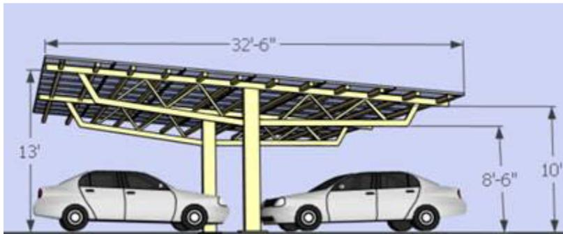
**Figure 6. A solar canopy design showing approximate dimensions of the structure (Structural Solar, 2013). Note that the width is not specified but the structure can accommodate a total of six cars.**
