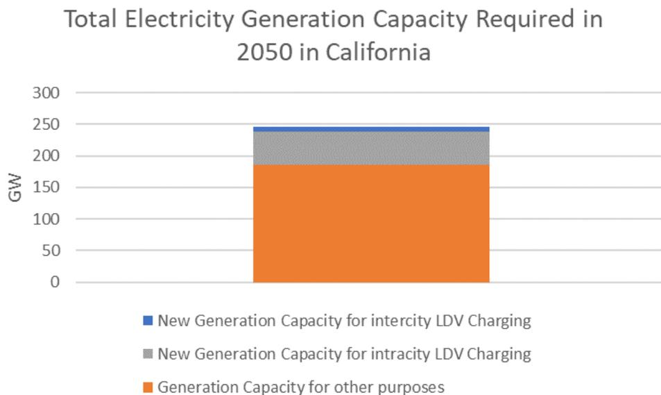
**Figure 26. Total installed generation capacity in 2050, to serve all electricity needs in California, including 30 million LDV BEVs. The fraction of capacity used for charging BEVs is shown as a stacked bar.**
