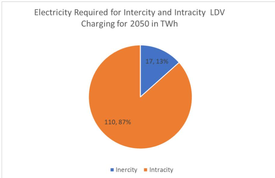
**Figure ES-2. Annual Electricity demand required for charging all 28 million BEV LDVs in 2050. Blue section is for intercity travel longer than 100 miles passing rest areas and orange section is for all other intracity travels.**
