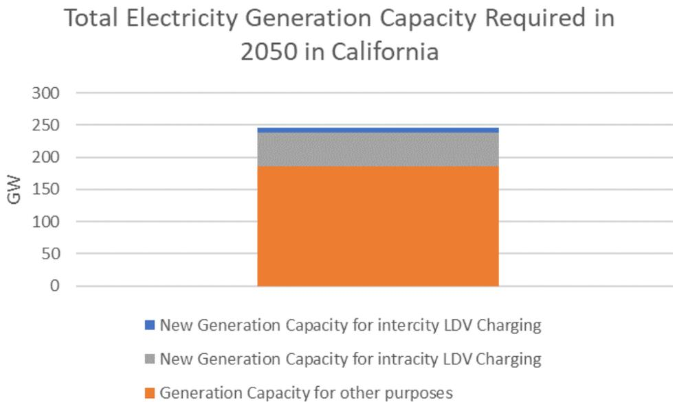
**Figure ES-3. Total installed generation capacity in 2050, to serve all electricity needs in California, including 30 million LDV BEVs. The fraction of capacity used for charging BEVs is shown as a stacked bar.**
