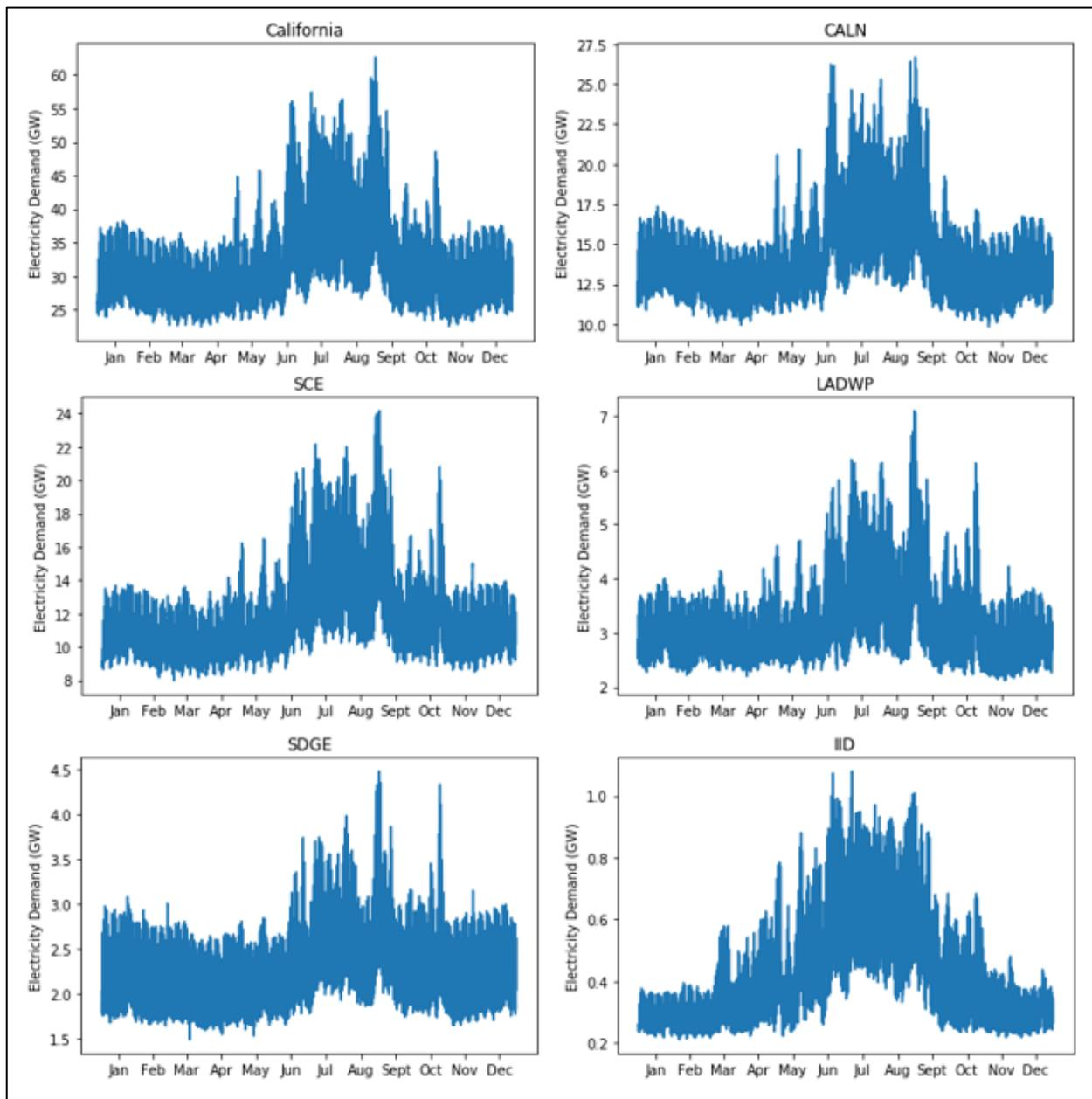
**Figure 4. Annual load profile for California and each of the five model regions in 2017. 2030 and 2050 load profiles have been calculated both endogenously by the optimization model based on hourly charging profile of increasing share of BEVs, and for all other sectors of the economy, exogenously based on electricity load forecasts for California.**
