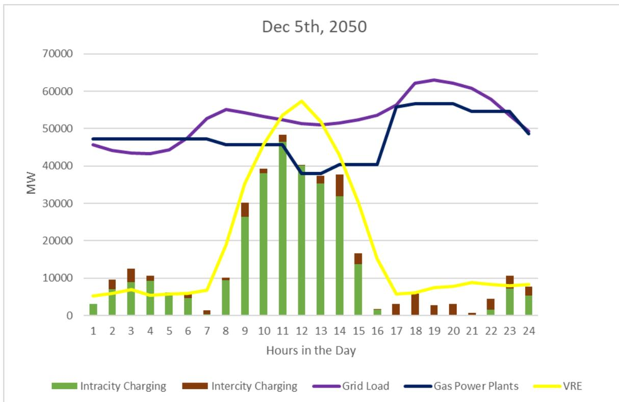
**Figure 23. Effect of charging on grid load in 2050 for a typical winter day. Brown bars show charging load for vehicles passing rest areas with trips longer than 100 miles range. Green bars show charging load from other vehicles mostly having intracity trips. The lowest line shows VRE, variable renewable energy (namely solar), the middle line Gas PP shows electricity production from natural gas, and the upper line shows the overall grid load.**
