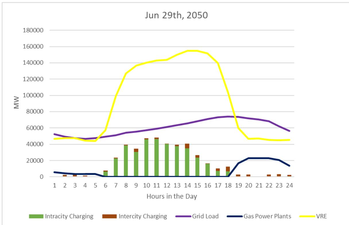
**Figure 22. Effect of charging on grid load in 2050 for a typical summer day. Brown bars show charging load for vehicles passing rest areas with trips longer than 100 miles range. Green bars show charging load from other vehicles mostly having intracity trips. The lower line shows electricity generated by gas power plants that has been flattened. Green and brown bars are stacked bars.**
