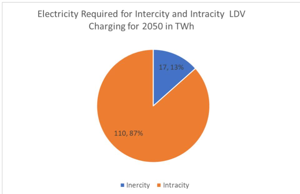
**Figure 25. Electricity demand required for charging all 28M BEV LDVs in 2050. Blue section is for intercity travels longer than 100 miles passing the rest areas and orange section is for all other intracity travels.**
