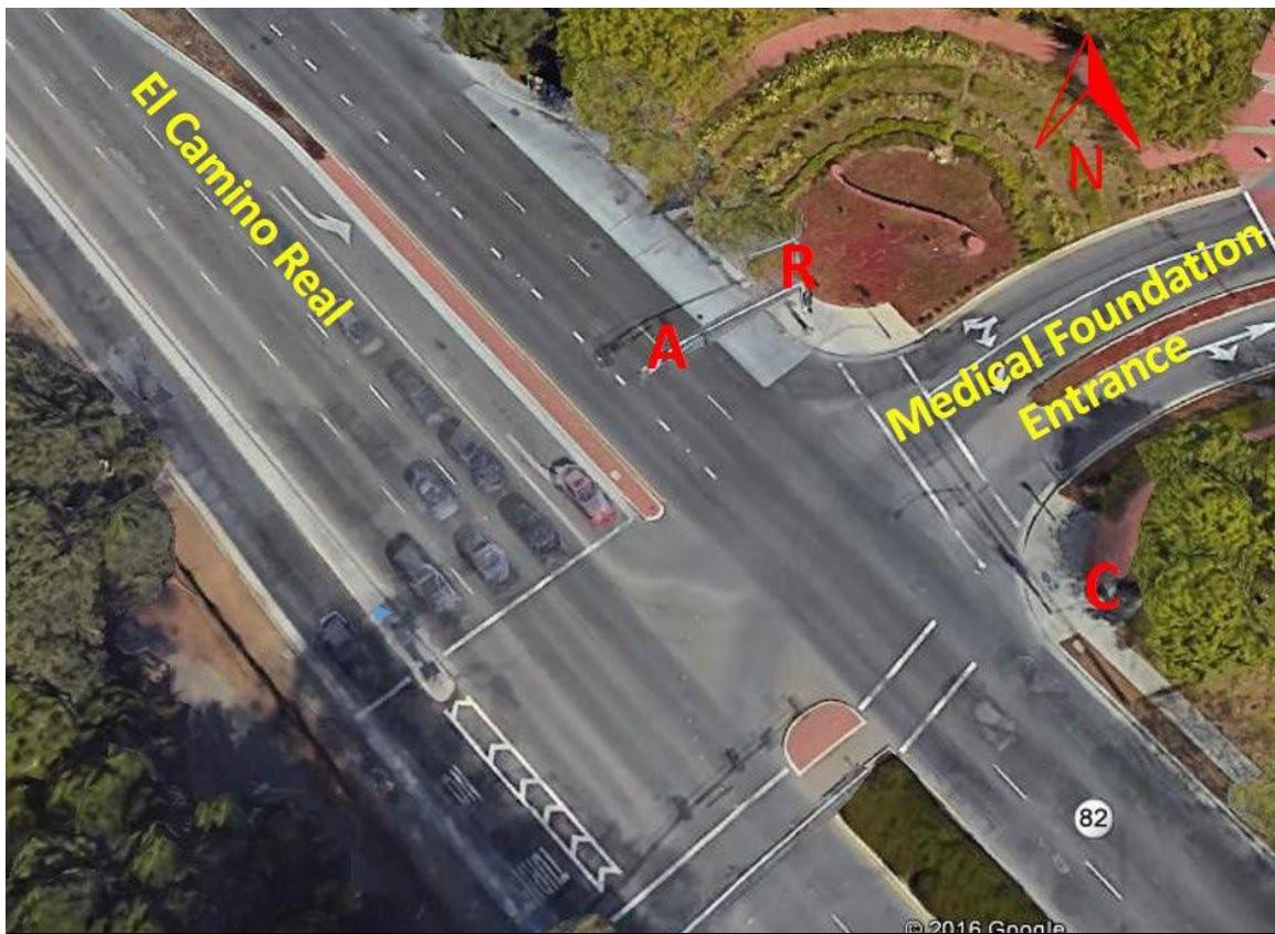
1. Install antenna (A) on mast arm with bracket.
