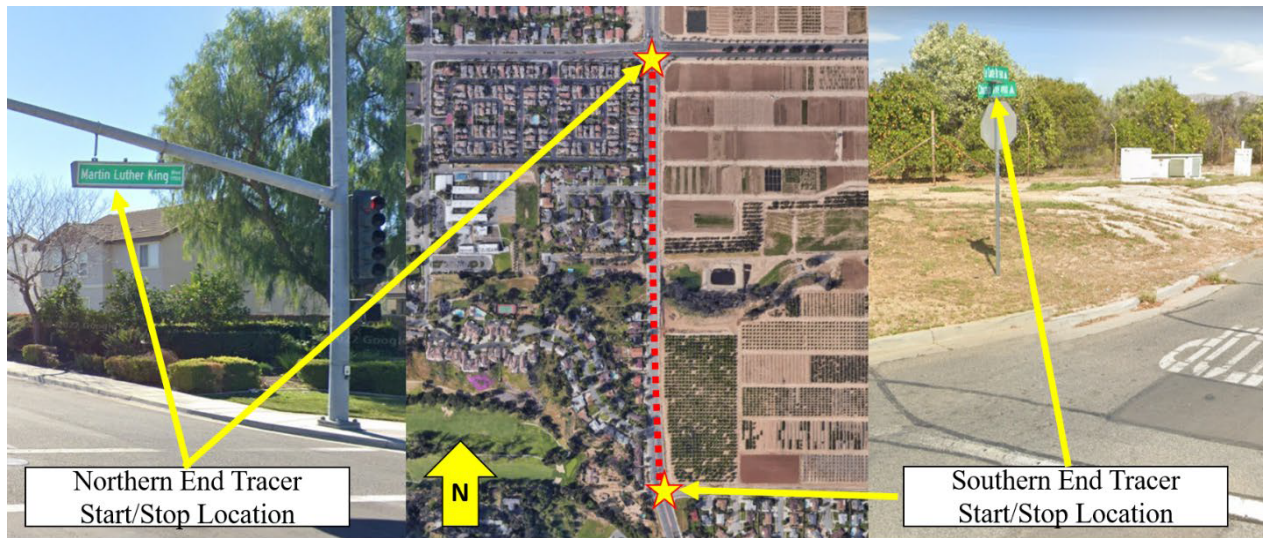
Figure 2-3 Tracer gas release start/stop locations at the no-barrier site.
