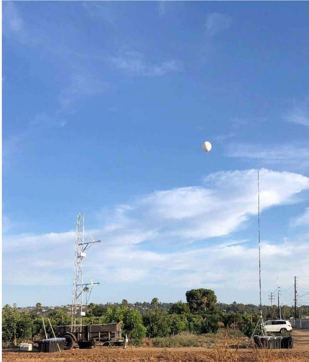
Figure 4-2 Pictures showing the meteorological tower, measurements tower and the helium balloon at the no barrier site.
