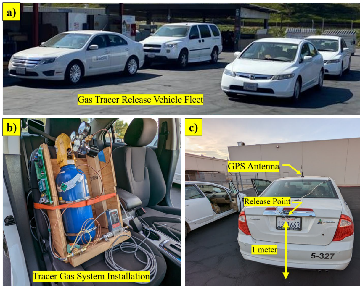
Figure 2-2 Vehicle equipped with tracer gas release system.
