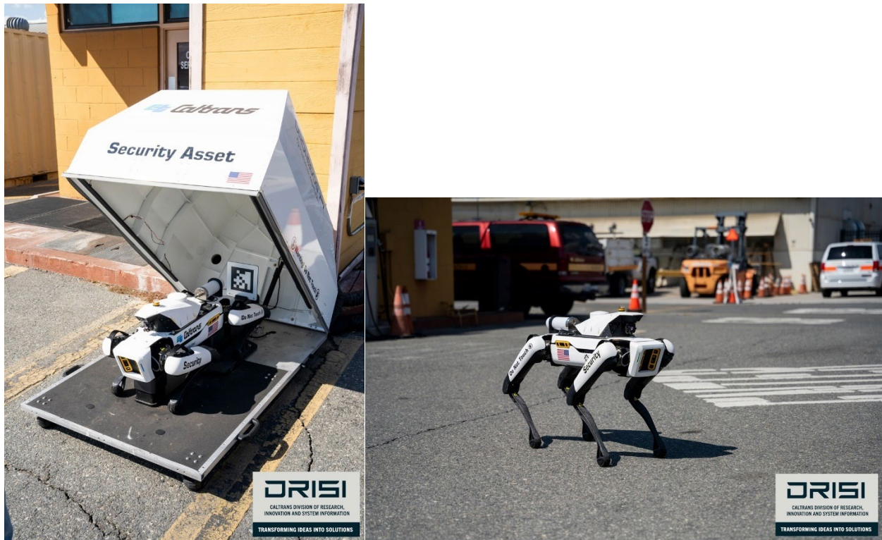
Figure A.2: Automated charging bay and weatherization DogHouse and the DroneDog equipped with Asylon's PupPack integrated with Boston Dynamics Spot (Asylon Robotics system deployed at Shop 8 - courtesy of DRISI)
