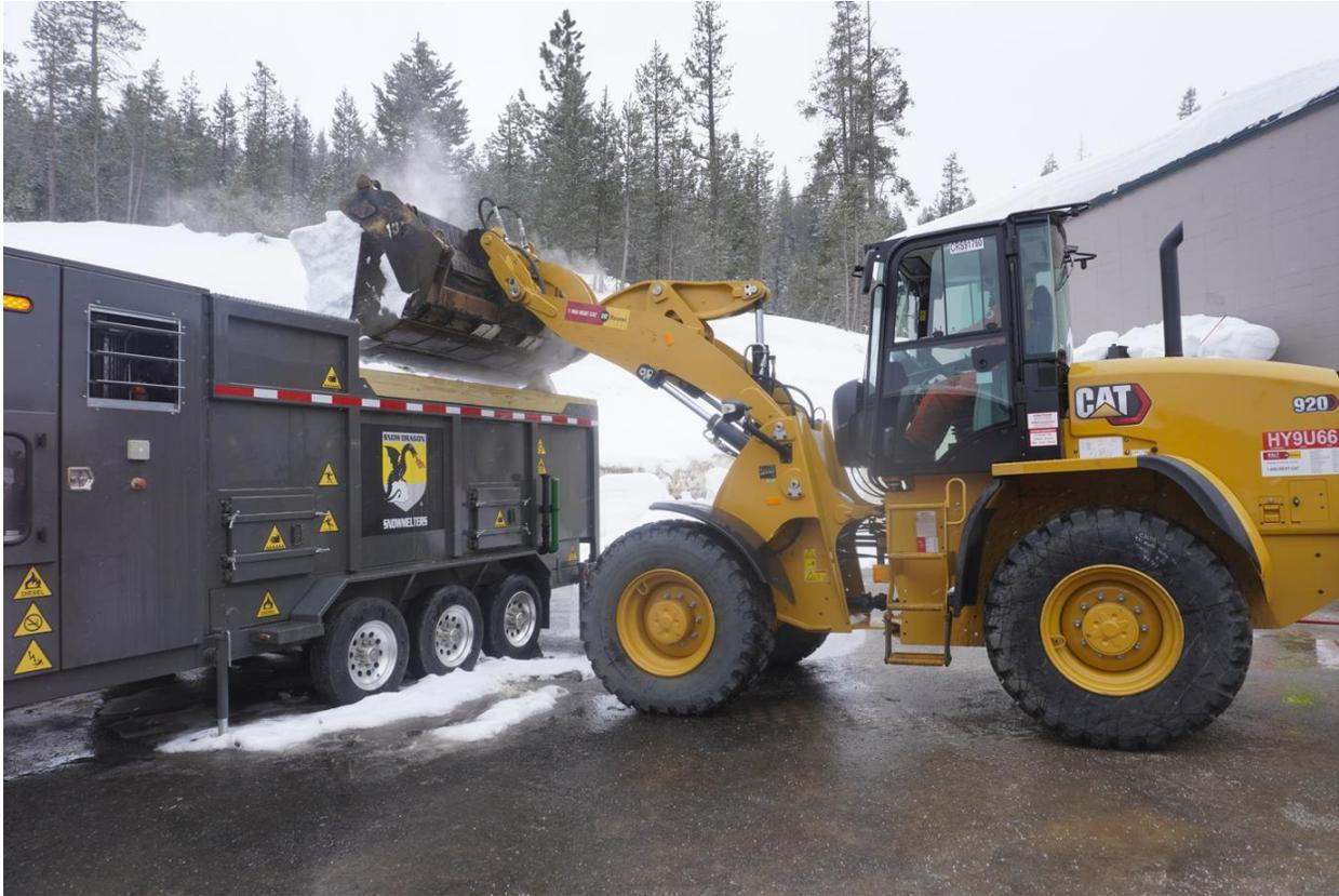
**Figure 4.4: Caltrans personnel trying out the Snow Dragon for the first time using the CAT loader to add snow**
