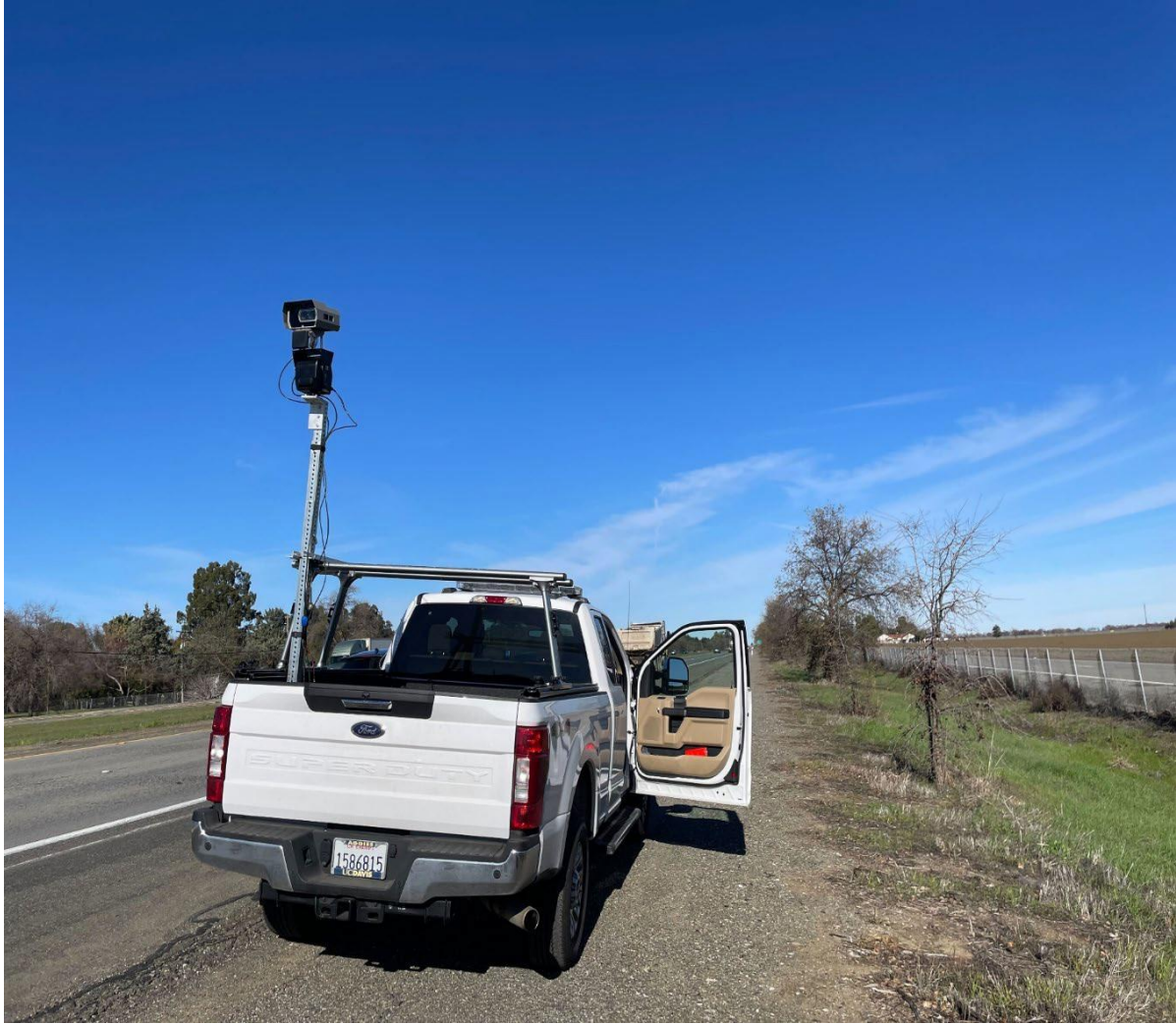
Figure 5.5: The camera orientation and vehicle placement on the shoulder.
